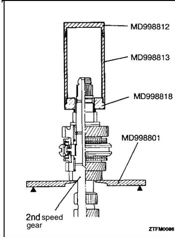
►F◄ INNER RING FOR REAR BEARING INSTALLATION
