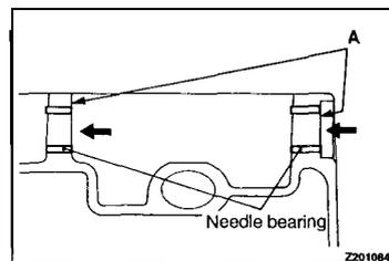
**REASSEMBLY SERVICE POINTS****▶A◀ NEEDLE BEARINGS INSTALLATION**
