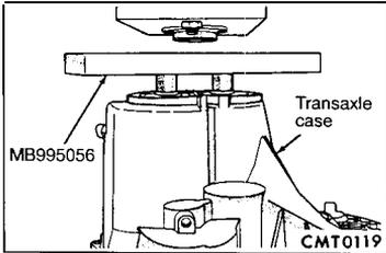
(14) Install bearing fixture (MB995056) onto transaxle end bearings. Verify tool is properly aligned to input and output shaft.
