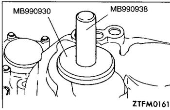
►D◄ **CENTER SHAFT OIL SEAL INSTALLATION**
