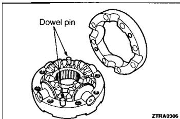
**REASSEMBLY SERVICE POINT****►A◄ CENTER DIFFERENTIAL CASE FRONT INSTALLATION**
