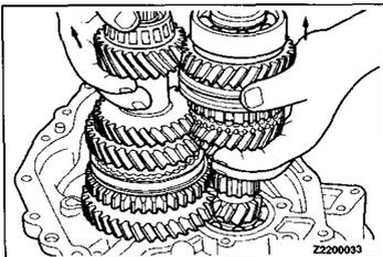
▶C▶ **INTERMEDIATE GEAR ASSEMBLY / INPUT SHAFT ASSEMBLY INSTALLATION**
