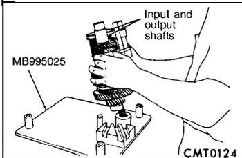
(21) Remove input and output shaft assemblies from bench fixture.
