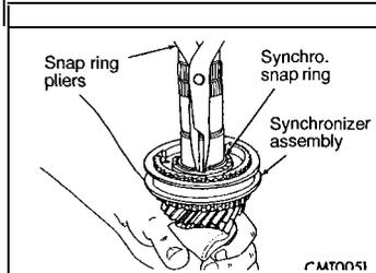
(9) Remove blocking ring. Remove 3/4 synchronizer hub retaining snap ring.
