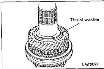
(4) Remove 4-5 gears split thrust washer ring.
