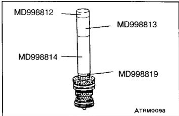
►E◄ **BALL BEARING INNER RACE INSTALLATION**
