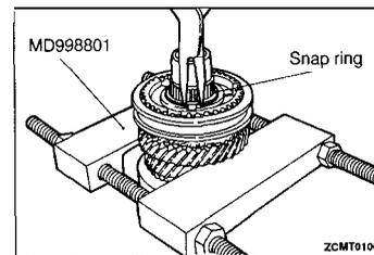
(12) Install 5th gear synchronizer snap ring.
