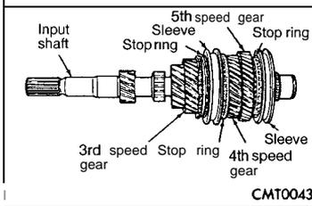
**INPUT SHAFT DISASSEMBLY**
