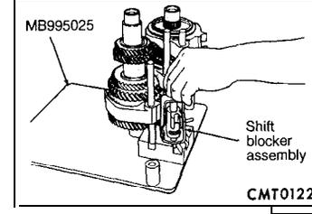
(19) Remove the shift blocker assembly from the bench fixture
