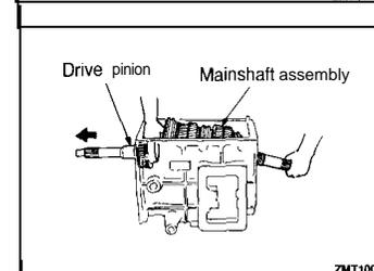
◀E▶ MAINSHAFT ASSEMBLY / DRIVE PINION REMOVAL
