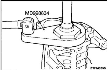
(2) Holding the driven bevel gear in a vice and using the special tool, remove the lock nut.
