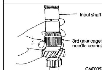
(11) Remove 3rd gear caged needle bearing. Check the caged needle bearing for a broken retention spring.
