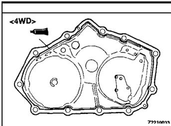
►R◄ SEALANT APPLICATION TO MACHINE SCREW
