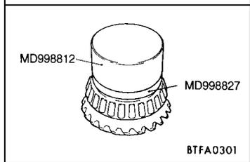
▶B◀ TAPER ROLLER BEARING INSTALLATION
