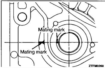
(3) Align the transfer case and drive bevel gear mating marks.
