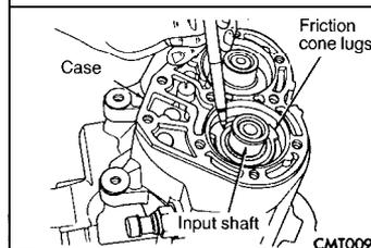
(10) Line up reverse brake friction cone lug to the slots in the gear case. Verify reverse brake shim is in position.
