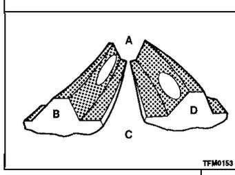
**3. Tooth contact pattern produced when driven bevel gear height is too small**
