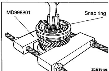
(1) Install MD998801 behind 5th speed gear. Remove snap ring at 5th synchronizer hub on input shaft.
