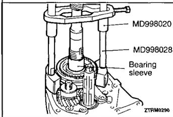
**◀C▶ BEARING SLEEVE REMOVAL**
