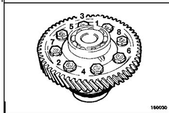
(2) Tighten to the specified torque while following the order given in the illustration.
