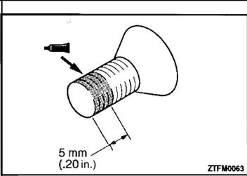
**►D◄ SEALANT APPLICATION TO BEARING RETAINER MOUNTING BOLT**
