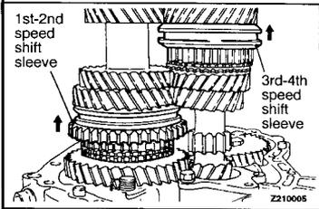
**►E◄ SHIFT RAIL ASSEMBLY INSTALLATION**
