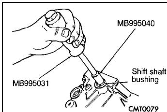
**SHIFTER SELECTOR SHAFT BUSHING****REMOVAL**
