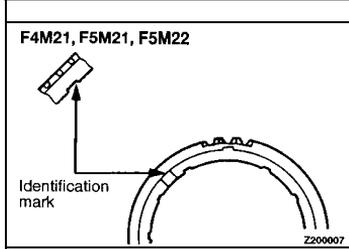
▶◀ **C** SYNCHRONIZER RINGS FOR 1ST SPEED GEAR, 2ND SPEED GEAR INSTALLATION
