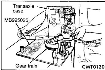
(17) Carefully remove transaxle case from the shaft assemblies and bench fixture.
