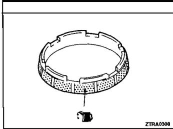
**REASSEMBLY SERVICE POINTS****▶A◀ INNER SYNCHRONIZER RING INSTALLATION**
