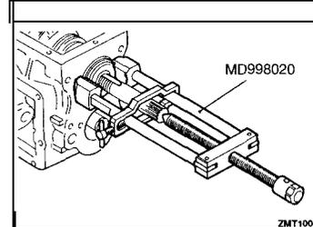
◀D▶ MAINSHAFT BALL BEARING / DRIVE PINION BALL BEARING REMOVAL
