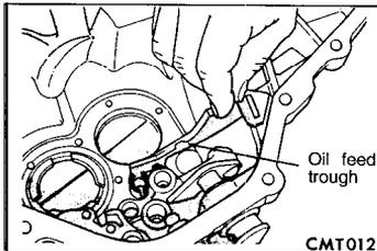
(18) Remove the reverse brake blocking ring, shim, reverse brake friction cone, bearing and race from the input shaft assembly.
