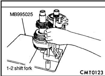
(20) Remove the 1-2 shift fork from the output shaft.
