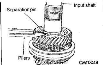
(6) Remove split thrust washer separation pin.
