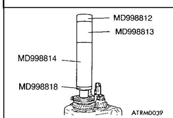
**►K◄ BEARING SLEEVE INSTALLATION**
