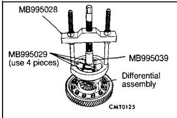
Install the bearing cone using the special tool.
