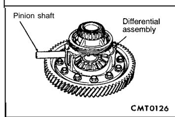
Remove the pinion shaft.
