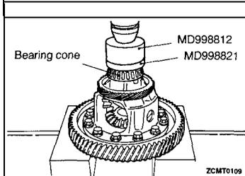
Install the differential bearing cone using the special tool.
