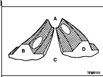
**2. Tooth contact pattern produced when drive bevel gear height is too large**
