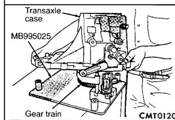
(9) Install gear case half over pallet fixture. Line up shift finger over 3/4 lug.
