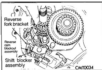
Remove reverse fork bracket and reverse cam blockout assembly.
