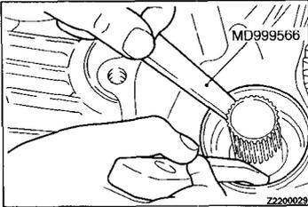
◀D▶ **BEARING OUTER RACE REMOVAL**
