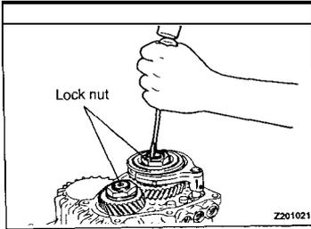
**DISASSEMBLY SERVICE POINTS****◀A▶ LOCK NUTS FOR INPUT SHAFT / INTERMEDIATE GEAR REMOVAL**
