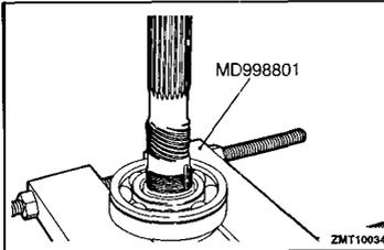
◀D▶ CLUTCH HUB (2-4WD) / BALL BEARING REMOVAL
