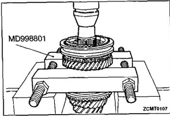
(2) Remove synchronizer and gear using shop press.
