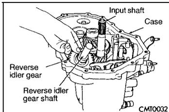
(18) Install reverse idler gear and shaft. Install bolt into shaft. Tighten bolt on shaft to 26 Nm (19 ft.lbs.) torque.
