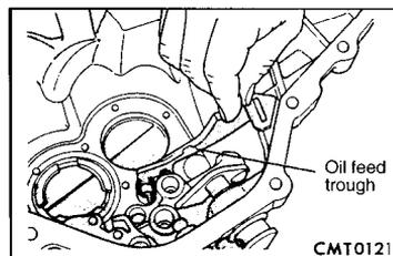
**REAR BEARING OIL FEED TROUGH****REMOVAL**
