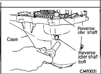
(7) Remove reverse idler shaft bolt.
