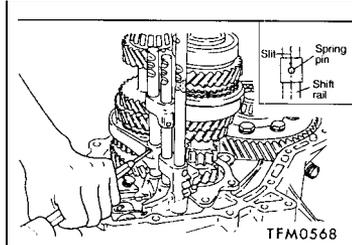
**►F◄ SPRING PINS FOR 1ST-2ND SPEED SHIFT FORK / 3RD-4TH SPEED SHIFT FORK INSTALLATION**
