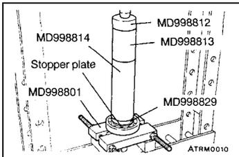
▶B▶ CLUTCH HUB (2-4WD) INSTALLATION
