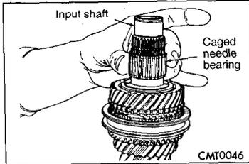
(3) Remove caged needle bearing.
