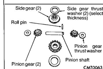
Assemble the differential side gears, pinion gears and pinion gears with the pinion gear washers. Rotate the assembly two full revolutions both clockwise and counterclockwise.
