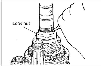
(2) Stake the area as shown in illustration of lock nut
