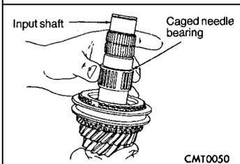
(8) Remove 4th gear caged needle bearing. Check the caged needle bearing for a broken retention spring.
