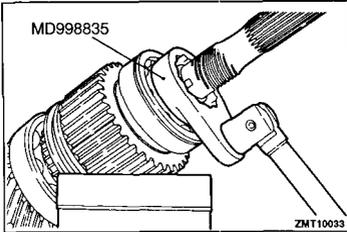
◀C▶ RADIAL BALL BEARING REMOVAL
