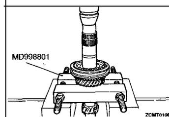
(10) Install input shaft in shop press. Using MD998801 to remove 3/4 synchronizer and 3rd gear.
