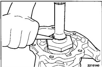
(2) Lock the lock nut at two positions.
