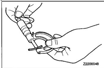
(5) Measure the thickness of the crushed solder with a micrometer and select and install a spacer of thickness that gives standard end play.
