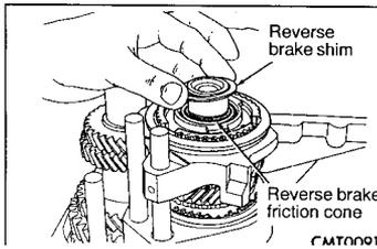
(8) Install reverse brake shim. Apply petroleum jelly to shim to hold in place.
