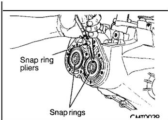
(12) Install shaft snap rings at input and output bearings.
