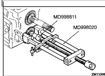
◀C▶ COUNTERSHAFT BALL BEARINGS REMOVAL
