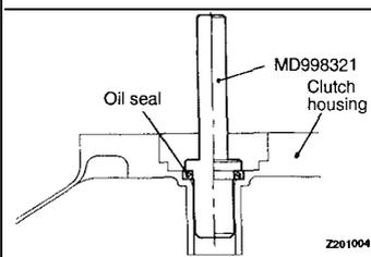
▶B▶ **OIL SEAL FOR INPUT SHAFT FRONT INSTALLATION**
