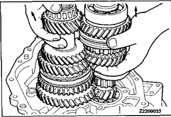
◀C▶ **INTERMEDIATE GEAR ASSEMBLY / INPUT SHAFT ASSEMBLY REMOVAL**
