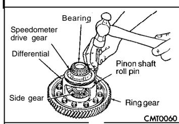
Remove the roll pin using a pin punch, etc.
