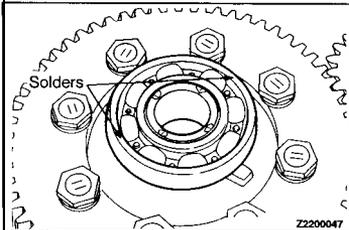
(2) Place two pieces of solder measuring about 10 mm (.39 in.) in length and 3 mm (.12 in.) in diameter on the bearing outer race as shown in illustration.
