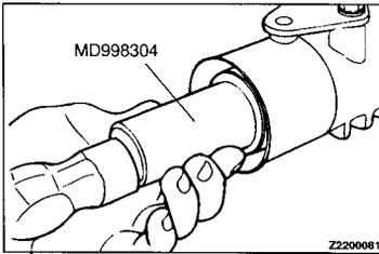
►B◄ **TRANSFER EXTENSION HOUSING OIL SEAL INSTALLATION**
