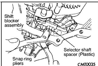
(9) Using snap ring pliers, remove selector shaft spacer.
