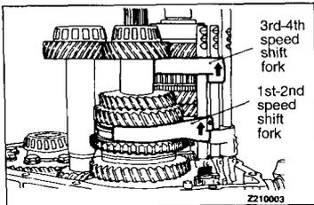
**◀B▶ SHIFT RAIL ASSEMBLY REMOVAL**
