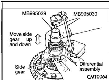
Set up dial indicator as shown and record end play. Rotate side gear 90 degrees and record another end play. Again, rotate side gear 90 degrees and record final end play. Using the smallest end play recorded, shim that side gear to within 0.25 mm (.0098 in.) to 0.33 mm (.0130 in.). The other side gear should be checked using the same procedure.
