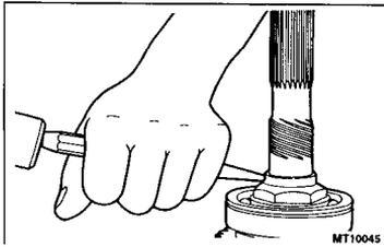
(2) Using a punch, crimp the lock nut at the groove in the rear output shaft.
