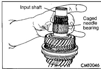
(10) Install 5th gear caged needle bearing.
