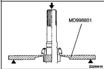
**◀B▶ BEARING SLEEVE FOR 5TH SPEED GEAR REMOVAL**
