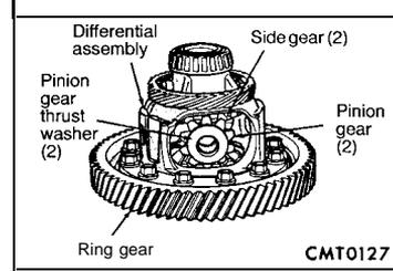
Remove the pinion gear, side gear and thrust washer.
