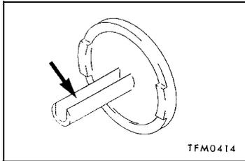
►C◄ **INPUT SHAFT REAR SEAL CAP INSTALLATION**
