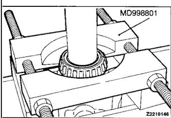
**DISASSEMBLY SERVICE POINTS****◀▶ TAPER ROLLER BEARINGS REMOVAL**
