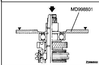
**◀C▶ 4TH SPEED GEAR | 3RD SPEED GEAR REMOVAL**
