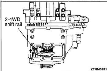
**◀B▶ H-L SHIFT RAIL / CHAIN COVER REMOVAL**
