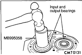
(11) Position input and output bearings on the shafts. Using MB995058, press input and output shaft bearings until they bottom into the case and against the shafts.
