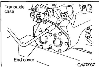
(13) Apply Loctite 18718 or equivalent to end cover outer edge and around bolt holes. Install end cover onto gear case. Tighten end cover bolts to 29 Nm (21 ft.lbs.) torque.
