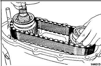
**◀C▶ REAR OUTPUT SHAFT ASSEMBLY / CHAIN / FRONT OUTPUT SHAFT ASSEMBLY REMOVAL**
