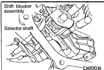
(16) Turn selector shaft into slot on shift blocker assembly.
