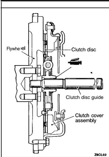
►◄ **CLUTCH DISC/CLUTCH COVER ASSEMBLY
