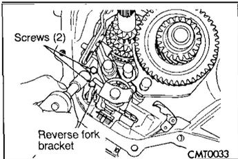
(8) Remove two screws retaining reverse fork bracket.
