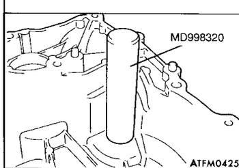
►E◄ **DRIVE SHAFT OIL SEAL INSTALLATION**
