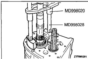
**◀D▶ MAINSHAFT CENTER BEARING REMOVAL**
