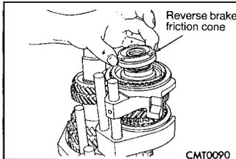
(7) Install reverse brake friction cone.
