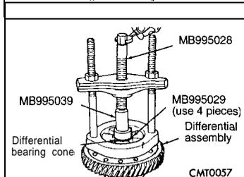
Install the bearing cone using the special tool.
