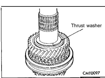
(9) Install split thrust washer retaining ring.
