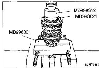
(11) Using MD998812, MD998821, install 5th speed gear and synchronizer. The 5th gear synchronizer hub has the letter "S" stamped on the top face of the hub. This designates that hub must be installed with the "S" facing upward.
