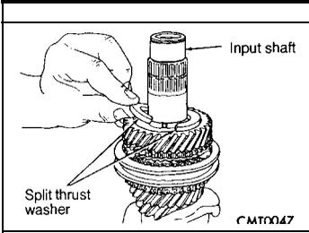
(8) Install split thrust washer onto input shaft.
