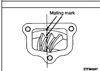
(6) With the mating marks aligned as in step (3), confirm that the transfer case and drive bevel gear mating marks are matched looking from the cover.
