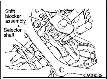
(10) Pull the selector shaft shift pin out of the slot in the blocker assembly. Turn selector shaft up and out of the way.
