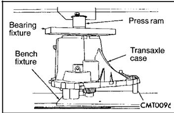
(15) Install transaxle gear case and bench fixture onto shop press. Press output and input shaft assemblies out of case.
