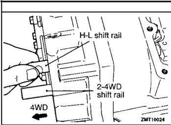
**DISASSEMBLY SERVICE POINTS****◀A▶ H-L SHIFT RAIL REMOVAL**
