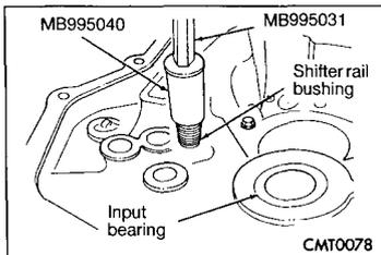
**SHIFTER RAIL BUSHINGS****REMOVAL**
