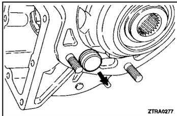
**◀D▶ COUNTER GEAR SHAFT REMOVAL**
