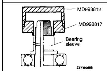
▶◀ BEARING SLEEVE FOR 5TH SPEED GEAR INSTALLATION
