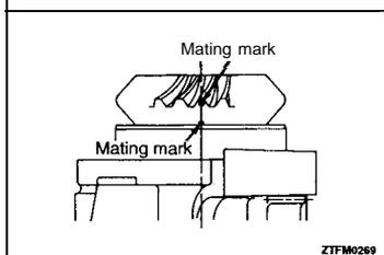
(4) Align the transfer case adapter and drive bevel gear mating marks.
