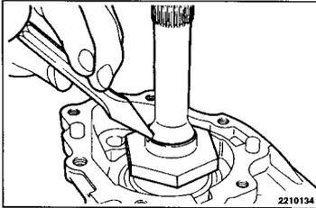
**DISASSEMBLY SERVICE POINTS****◀A▶ LOCK NUT REMOVAL**
