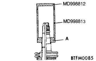
**▶C◀ BEARING SLEEVE FOR 4TH SPEED GEAR INSTALLATION**
