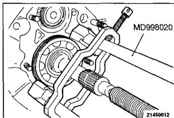
**◀E▶ MAINDRIVE GEAR BEARING REMOVAL**
