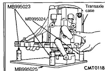
(13) Using bench fixture and shims provided (MB995023, MB995024, MB995025), turn transaxle over. Install transaxle onto bench fixture. Verify shim spacers are in position on bench fixture. Install transaxle into shop press.
