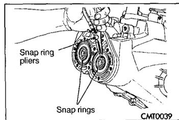
(12) Remove two snap rings retaining the output shaft and the input shaft to the bearing.
