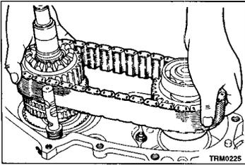
**◀F▶ 2-4 SYNCHRONIZER ASSEMBLY | CHAIN | FRONT OUTPUT SHAFT ASSEMBLY REMOVAL**
