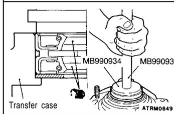
**▶B◀ OIL SEAL (INPUT GEAR) INSTALLATION**
