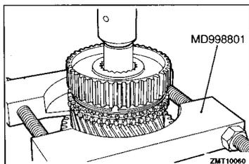
**DISASSEMBLY SERVICE POINT****◀A▶ SYNCHRONIZER HUB REMOVAL**
