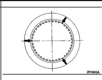
(2) Install the synchronizer sleeve with its low tooth portions at synchronizer key positions.
