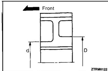
**►D◀ SYNCHRONIZER HUB FOR THIRD AND FOURTH SPEED INSTALLATION**
