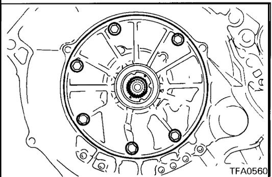
30. Remove oil pump installation bolts.
