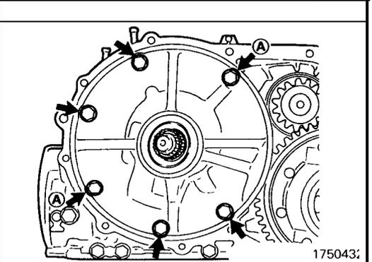
(17) Remove the six oil pump mounting bolts indicated by arrows.
