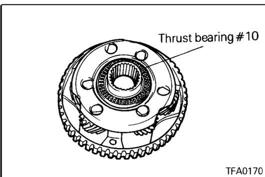
14. Apply a coating of petrolatum to thrust bearing #10 and attach to the planetary carrier.
