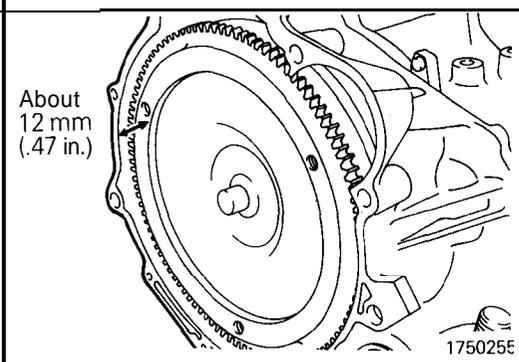
(90) After applying automatic transmission fluid to the outside surface of the oil pump-side cylindrical portion of the torque converter, install the torque converter carefully so as not to give damage to the oil seal lip. Make certain that the torque converter is in mesh with the oil pump drive gear.
