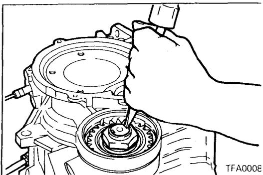
(48) Straighten the locking tab of the transfer shaft lock nut where it is bent.
