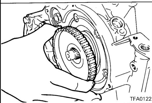
23. Remove the end clutch hub.
