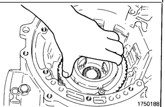
(24) Mount the planetary carrier on the case.
