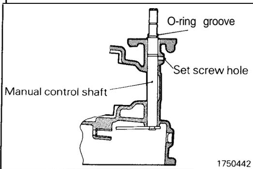
(72) Install the parking sprag rod to the manual control shaft. Then, insert the shaft in the transaxle as shown in the illustration. In doing this work, do not install O-ring in the O-ring groove.
