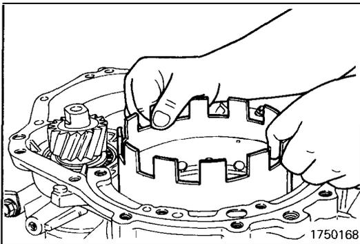
(42) When putting the kickdown drum in the kickdown band, engage the splines of the kickdown drum with those of the reverse sun gear. Place the kickdown band on the kickdown drum and tighten the kickdown servo adjusting screw to keep the band in position.
