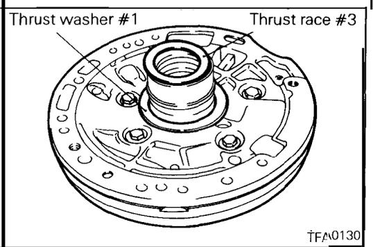
49. Adhere thrust race #3 and thrust washer #1 to the back of the oil pump with petrolatum.
