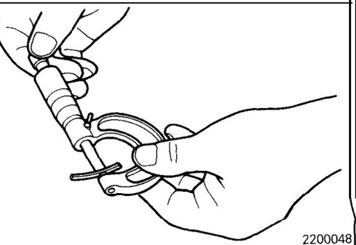
66. Measure the thickness of the crushed solder with a micrometer and adjust by selecting a spacer with a thickness that will provide the standard value for the end play and preload.
