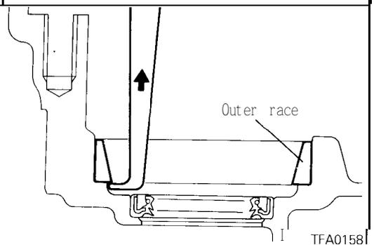
59. Using a sliding hammer or similar tool, remove the outer race.
