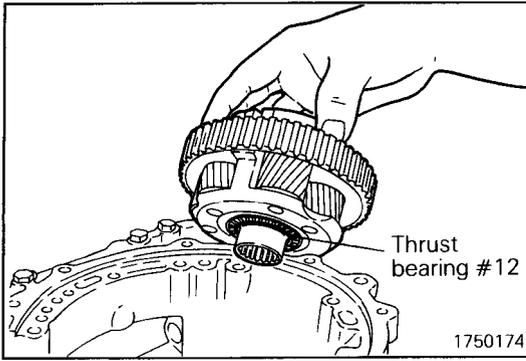
(35) Remove the planetary gear set and thrust bearing #12.
