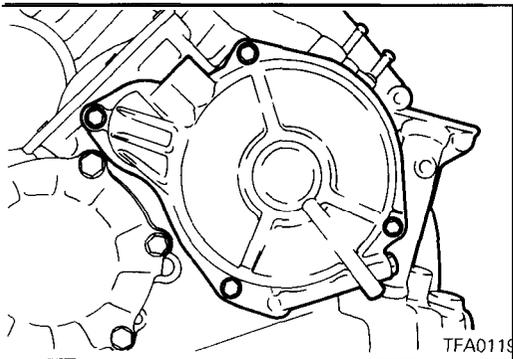
61. Install the end clutch cover and tighten the bolts to the specified torque.
