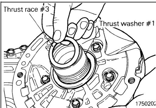
(47) Attach thrust race #3 and thrust washer #1 to the rear end face of the oil pump with petrolatum jelly.
