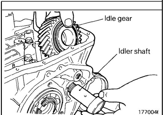
(43) Pull out the transfer idler shaft. Remove the transfer idle gear and the two bearing inner races from inside the case.
