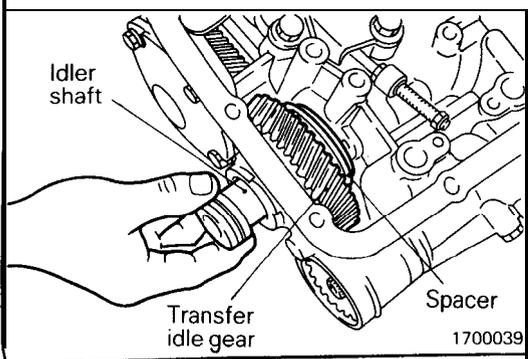
(39) Pull out the transfer idler gear shaft, and remove the transfer idler gear, the two bearing inner races, and the spacer.
