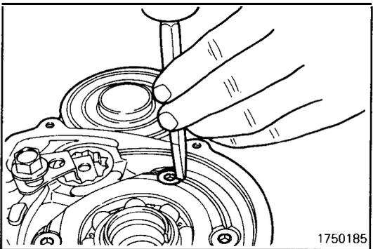
(22) Lock the screw head in place using a chisel.
