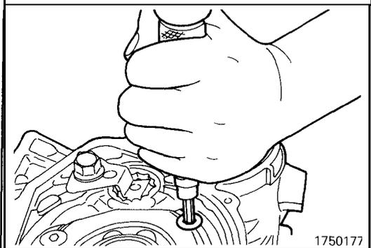
(40) Using an impact driver, loosen the screws and remove the bearing retainer.
