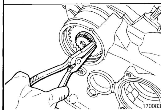
(43) Remove the snap ring from the transfer shaft.
