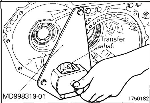
(14) Mount the special tool on the transmission case to support the transfer shaft.
