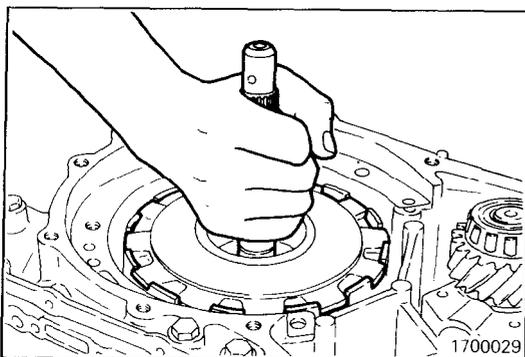
(22) Grasp and raise the input shaft to remove both the front and rear clutch assemblies together.
