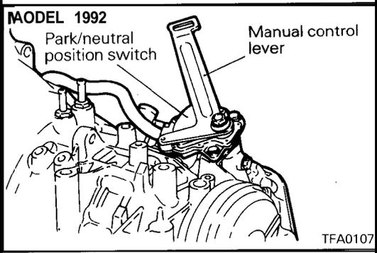
6. Remove manual control lever then remove park/neutral position switch (PNP switch).
