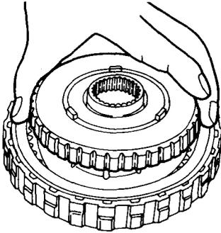
57. Install the end clutch hub on the end clutch assembly.
