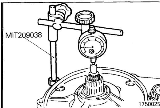
(51) Measure the end play of the input shaft. If the measurement is out of specification, replace thrust race #3 and thrust washer #1 to meet the specification.
