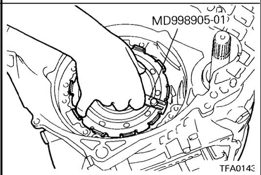
33. Mount the special tool on the center support, install 2 new O-rings and push into the transaxle case.
