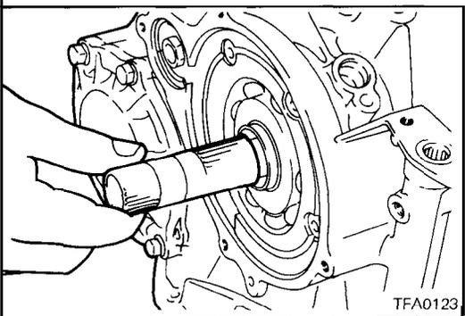
55. Insert the end clutch shaft from the end with the long spline.
