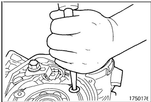
(39) Sealant has been applied to the threads of the screws on the bearing retainer. Tap the screw heads so the screws can be easily loosened.
