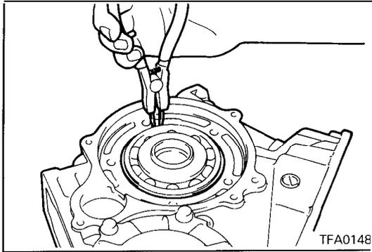
11. Insert the output flange into the case and install a snap ring around the bearing.
