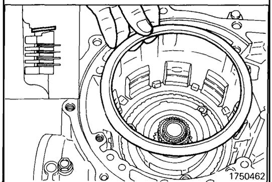
(27) Apply petrolatum jelly to the wave spring and attach the wave spring to the center support.
