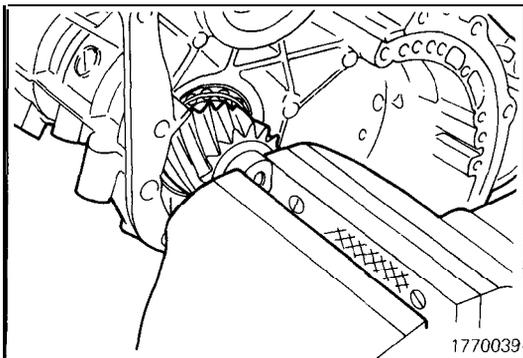
(49)Secure the transfer shaft on the end of the converter housing.
