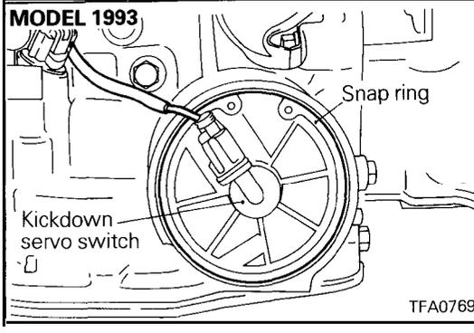
(7) Snap off the snap ring and remove the kickdown servo switch.,
