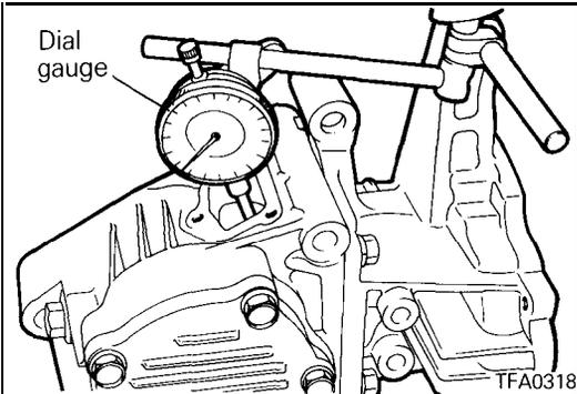
(6) Check to see if the drive bevel gear and driven bevel backlash is as specified.
