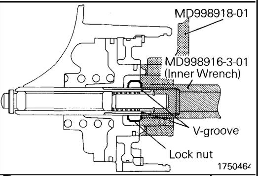
84. Install the pulse generator A and B.
