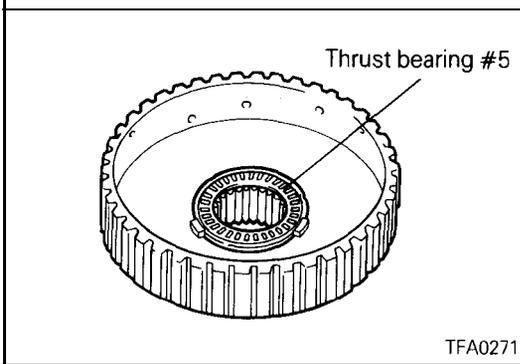
43. Install thrust bearing #5 on the rear clutch hub.
