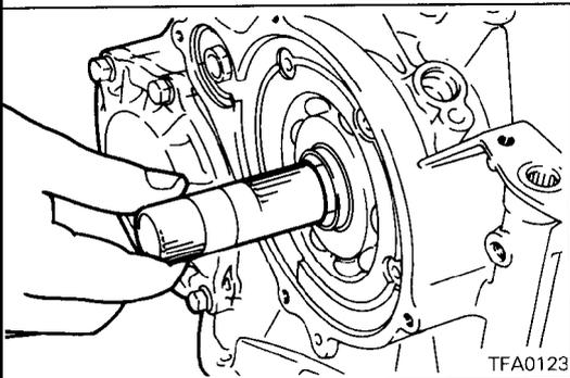
25. Pull out the end clutch shaft
