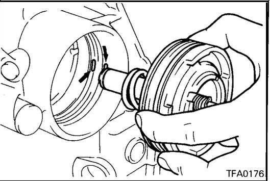
38. Install the kickdown servo spring, piston and sleeve.
