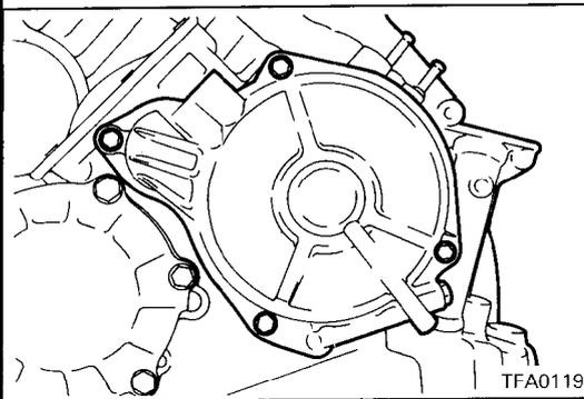
20. Take out the end clutch cover installation bolts, then remove the cover holder and end clutch cover.
