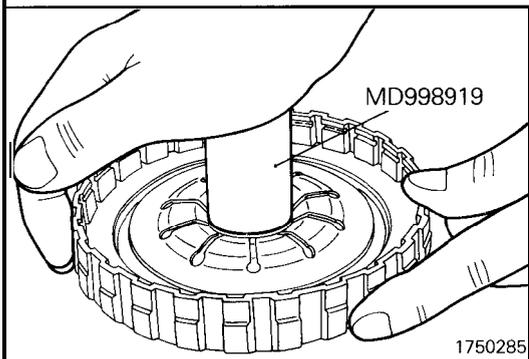
**REASSEMBLY SERVICE POINTS****◆A◆ SNAP RING INSTALLATION**
