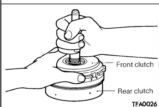
(44) Mate the rear clutch assembly with the front clutch assembly.
