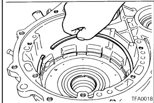
(31) Install the snap ring for the center support.
