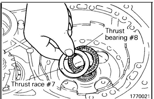
(28) Remove thrust race #7 and thrust bearing #8.
