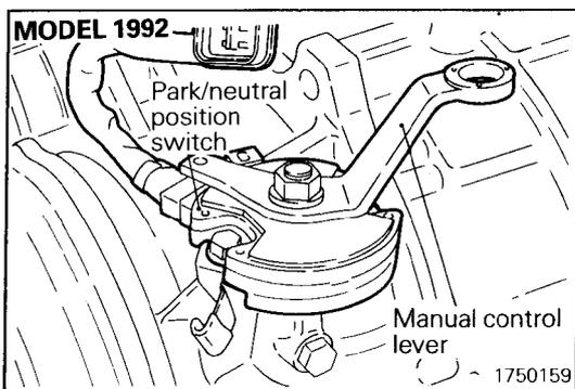
(86) Install the park/neutral position switch and manual control lever, and tighten the manual control lever nut to the specified torque.
