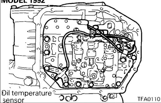
9. Remove the 10 valve body mounting bolts.
