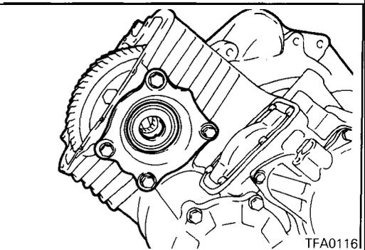
64. Install the differential rear bearing retainer and tighten the bolts to the specified torque.
