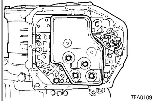
81. Install the magnets in the oil pan and install the oil pan.
