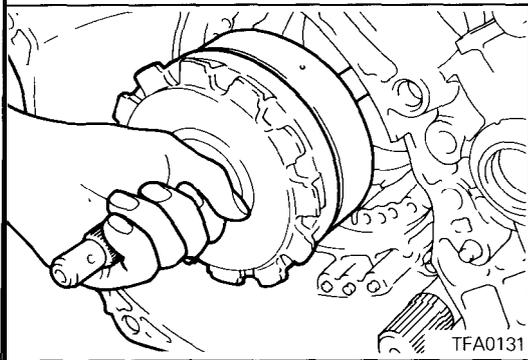
33. Hold the input shaft and remove the front clutch assembly and rear clutch assembly together.
