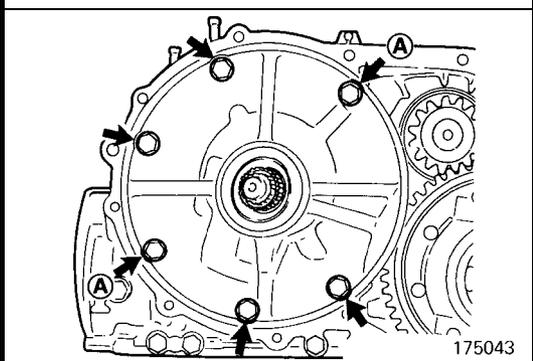
(20) Remove the six oil pump mounting bolts indicated by arrows.
