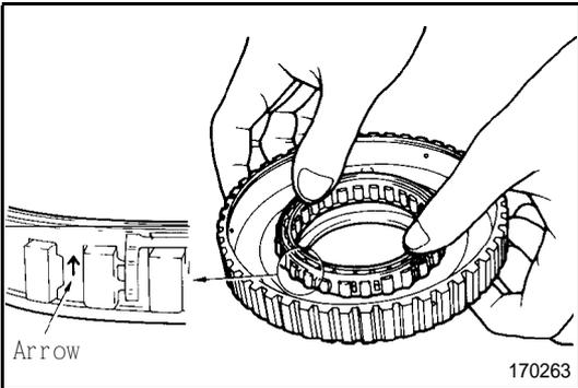
**◆B◆ ONE-WAY CLUTCH INSTALLATION**
