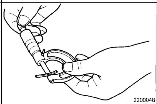
54. Measure the thickness of the crushed solder with a micrometer and adjust by selecting a spacer with a thickness that will provide the standard value for the end play and preload.
