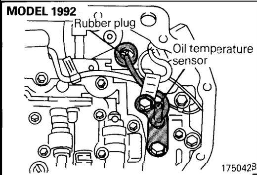
(10) Remove the oil temperature sensor bracket mounting bolts, and remove the oil temperature sensor from its bracket. Using a screwdriver, push out the rubber plug, working from inside the case, and remove the oil temperature sensor from the case.
