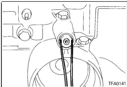
43. Remove the plug, then remove the air exhaust plug.
