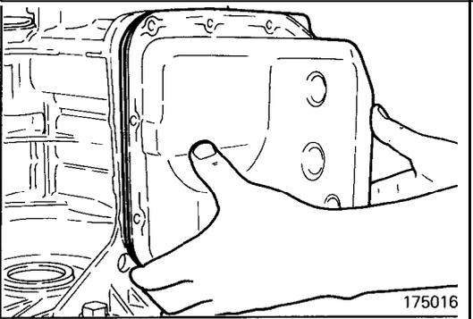
(76) Clean the gasket surfaces of both the transaxle case and oil pan. Using a new oil pan gasket, install the oil pan by tightening the 12 bolts to the specified torque.
