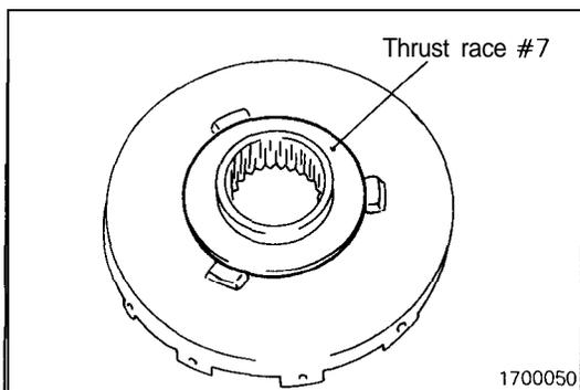
(40) Apply petrolatum jelly to thrust race #7 and attach the thrust race to the rear clutch hub.
