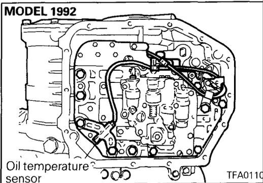
9. Remove the 10 valve body mounting bolts.
