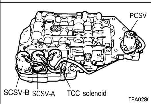
**SOLENOID VALVE ASSEMBLY INSTALLATION**
