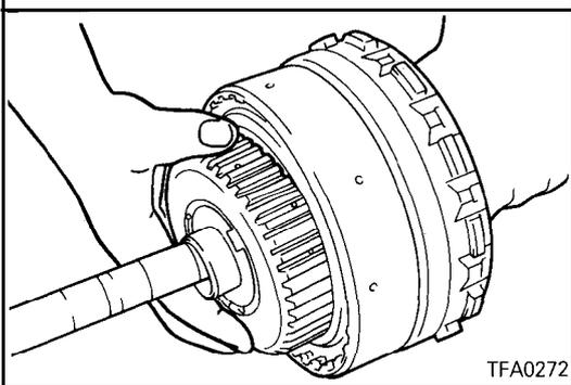
32. Install the rear clutch hub on the rear clutch.
