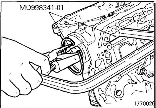
(31) Using the special tools, push in the kickdown servo and remove the snap ring.
