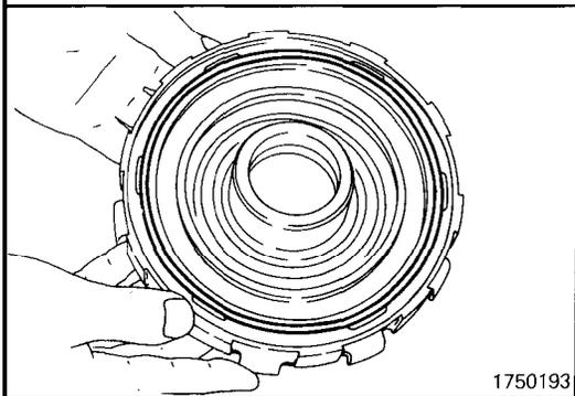
20. Apply a coating of petrolatum jelly to the wave spring and attach it to the center support.
