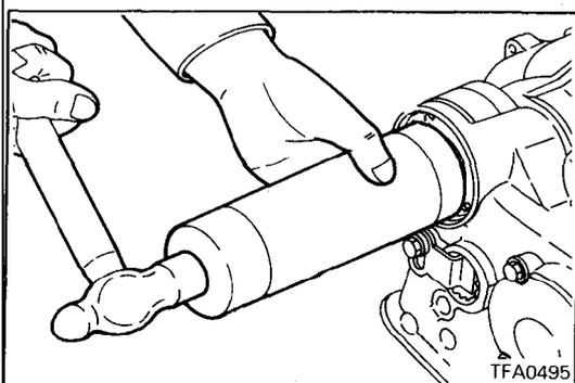
(17) Use the special tool to install the transfer driven gear on the transfer shaft.
