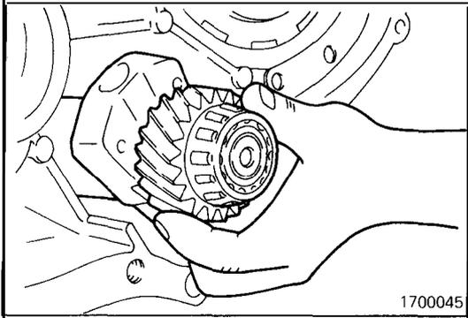
(13) Insert the transfer shaft in the case.
