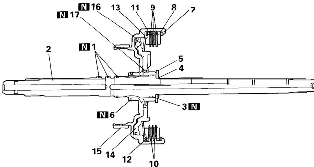
DISASSEMBLY AND REASSEMBLY – F4A33, W4A33
