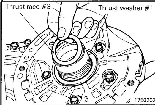
(51) Attach thrust race #3 and thrust washer #1 on the rear end face of the oil pump with petrolatum jelly.
