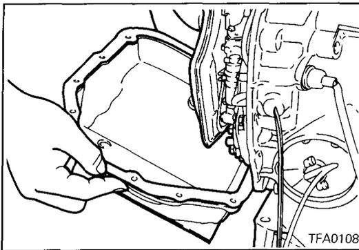
7. Remove the oil pan, magnets and gasket,
