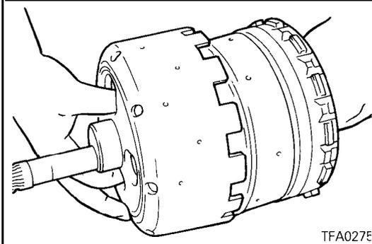
35. Install the clutch assembly in the kickdown drum
