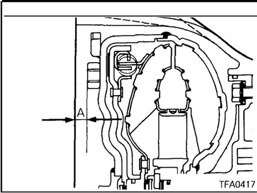
78. Coat the oil pump drive hub with automatic transmission fluid and install the torque converter. Push in firmly so that dimension A in the diagram is the standard value.
