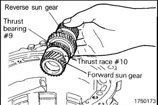
(36) Remove reverse sun gear, thrust bearing #9, thrust race #10 and forward sun gear together.
