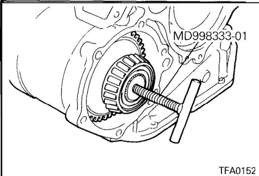
15. Install the special tool in the center differential and install the center differential in the transaxle case.
