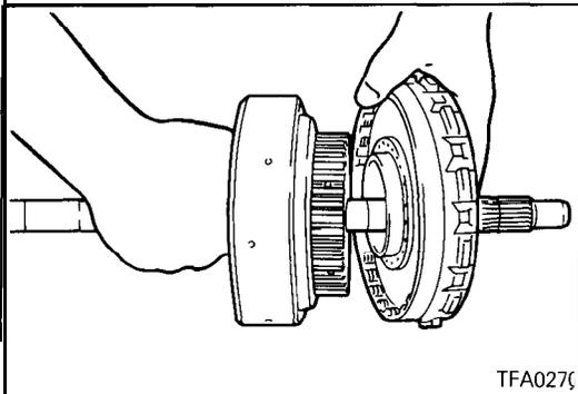
42. Combine the rear clutch assembly and the front clutch assembly.
