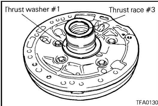
32. Remove thrust washer #1 and thrust race #3.
