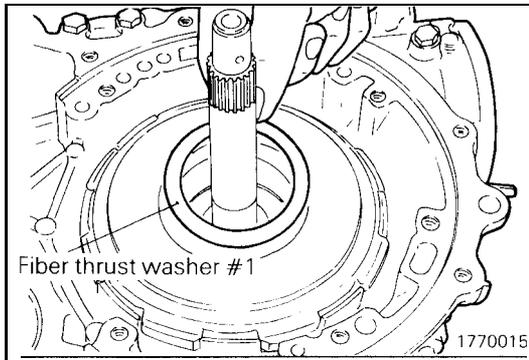
(24) Remove fiber thrust washer #1
