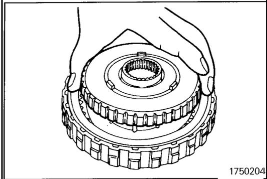
45. Install the end clutch hub on the end clutch assembly.
