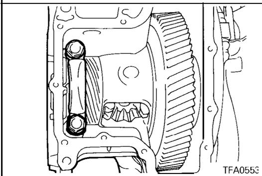
16. Remove the differential cover and gasket.
