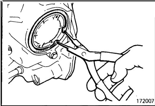
(36) Insert the kickdown servo sleeve in the transaxle case and install the snap ring.
