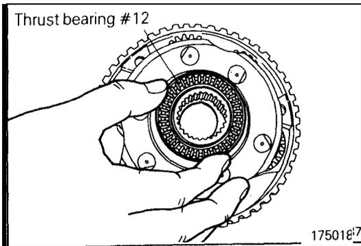
(20) Apply petrolatum jelly to thrust bearing #12 and secure the bearing on the planetary carrier.
