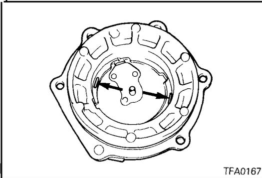
16. Place solder with a length approximately 10 mm (.39 in.) and diameter of 1.6 mm (.06 in.) on the output bearing retainer at the position shown in the diagram and install the outer race.
