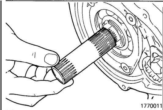
(18) Pull out the end clutch shaft.
