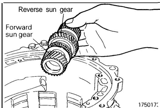
(34) Remove reverse sun gear, thrust bearing #9, thrust race #10 and forward sun gear together.
