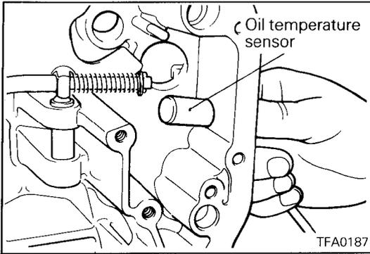
62. Insert the oil temperature sensor into the case.
