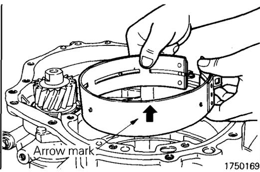
(41) Install the kickdown band; attach the ends of the band to the ends of the anchor rod and servo piston rod.
