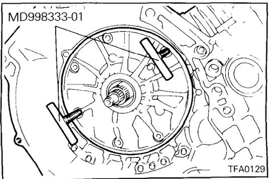
50. Use the special tool to install a new oil pump gasket and oil pump assembly.
