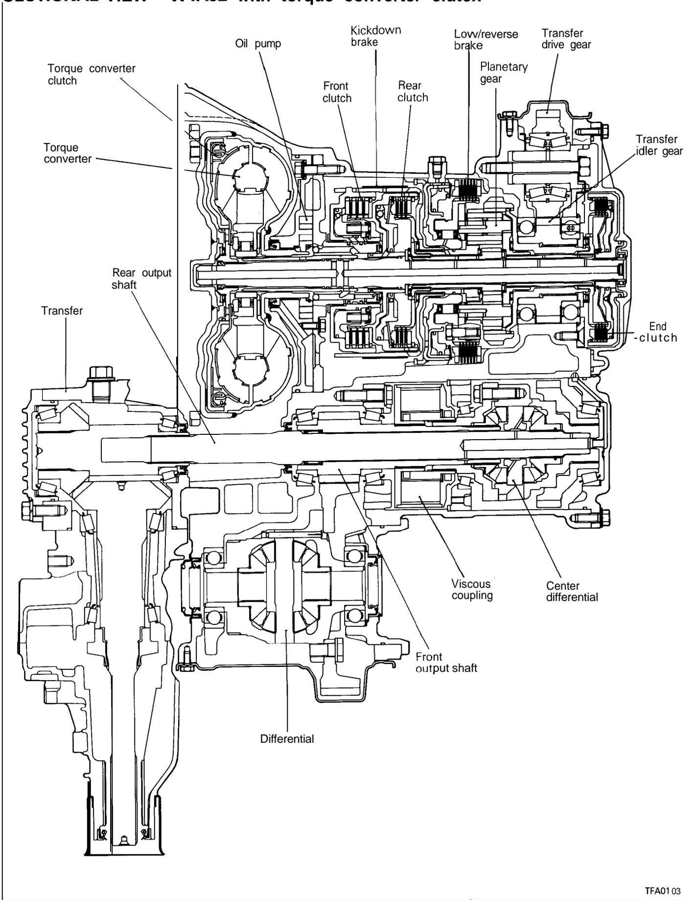
SECTIONAL VIEW – W4A33 without torque converter clutch
