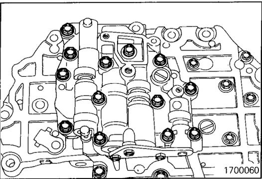
(2) Secure the lower valve body with the 13 bolts. Remove the special tools.
