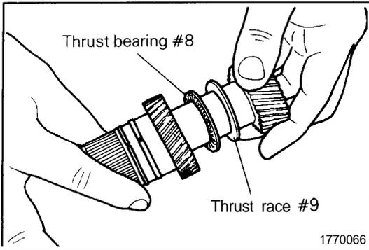
16. Assemble the forward sun gear, thrust race #9, thrust bearing #8 and reverse sun gear.
