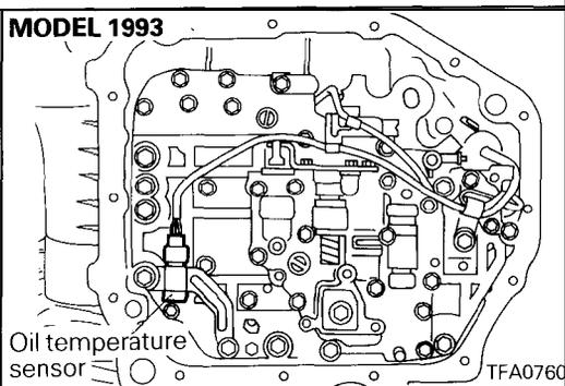
11. Press the finger of the solenoid valve harness grommet, push the grommet into the case and remove the valve body assembly.
