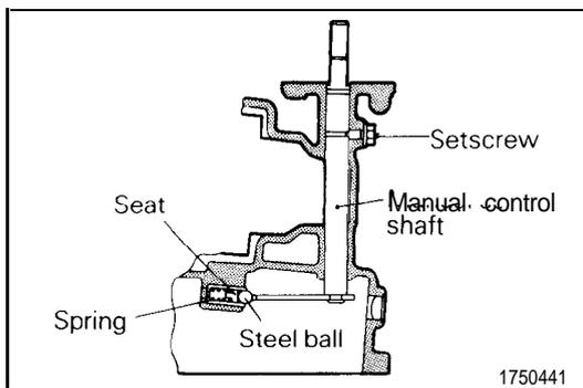
(73) After installing a new O-ring on the manual control shaft assembly, draw the shaft back into the case, then install the set screw and gasket. Also install the detent steel ball, seat and spring at the same time.
