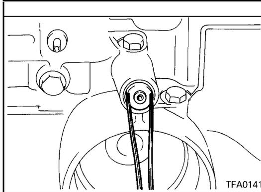
24. Install the air exhaust plug, and then install the plug.
