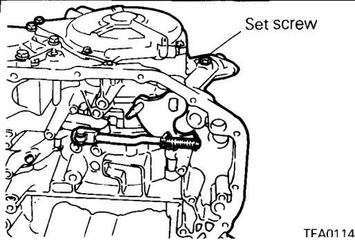
14. Remove the set screw of the manual control shaft and remove the manual control shaft assembly.
