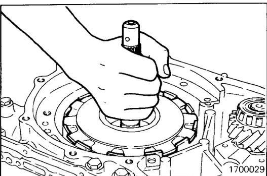
(45) Install the clutch assembly.
