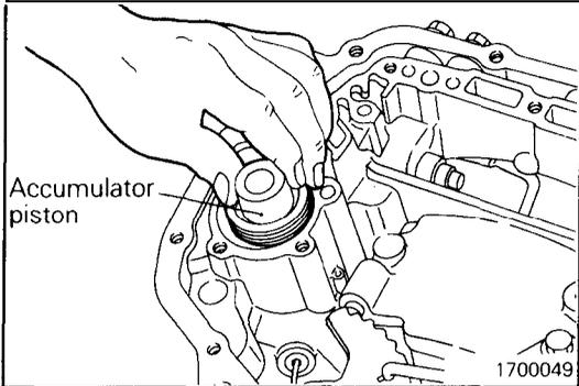
(68) Install new seal rings in the groove of the accumulator piston and coat the rings with automatic transmission fluid.
