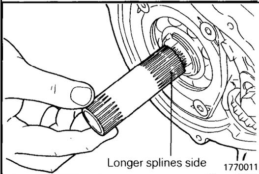
(65) Install the end clutch shaft, inserting the end that has the longer splines first.
