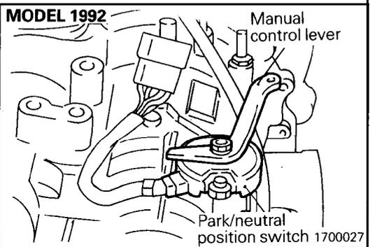
(77) Install the park/neutral position switch (PNP switch) and manual control lever, and tighten the manual control lever nut to the specified torque.
