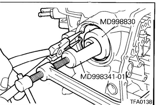
39. Use the special tool to push in the kickdown servo piston and sleeve, and then install a snap ring.
