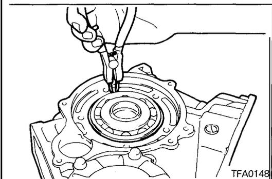
50. Remove the snap ring and then remove the output flange assembly.
