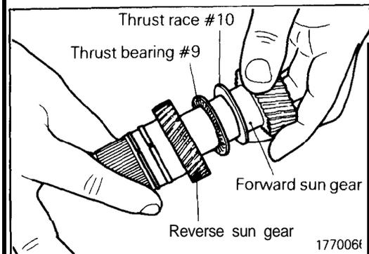
(22) Attach thrust race #10 and thrust bearing #9 to the forward sun gear. Then, assemble the reverse sun gear.
