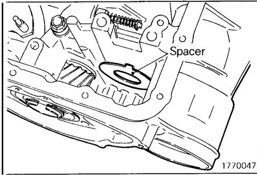
(14) Apply petrolatum jelly to the spacer and attach the spacer to the case.
