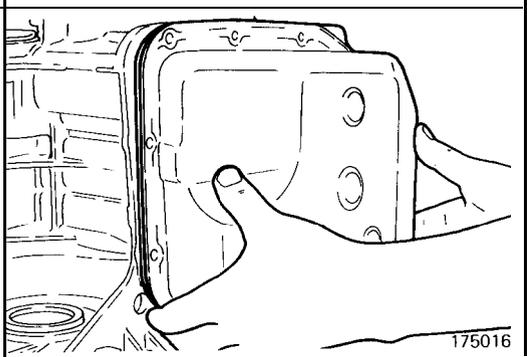
(9) Remove the oil pan and oil pan gasket.
