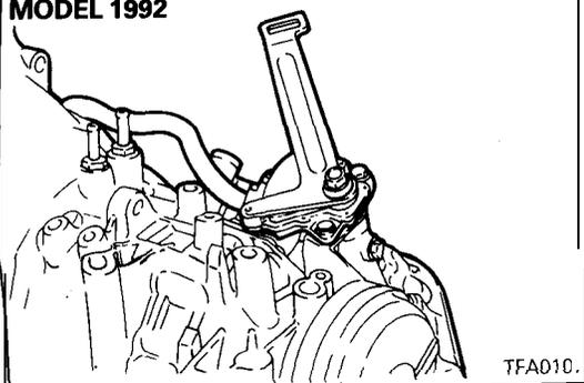
82. Install park/neutral position switch (PNP switch) and manual control lever.
