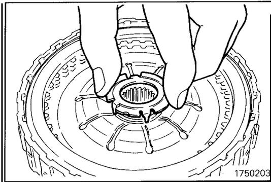
44. Fit the thrust washer on the return spring of the end clutch.
