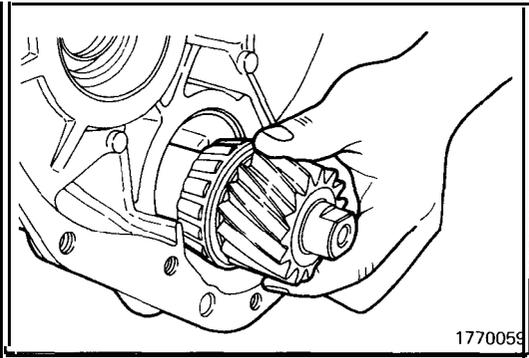
(3) Insert the transfer shaft in the case.
