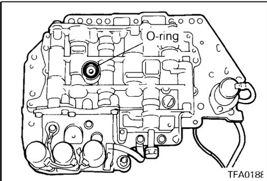
63. Install an O-ring in the O-ring groove at the top of the valve body assembly.
