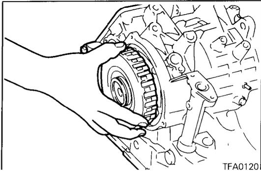
21. Remove the end clutch assembly.
