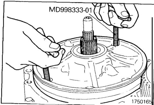
(19) Grasping the special tools, remove the oil pump. Then, remove the gasket.
