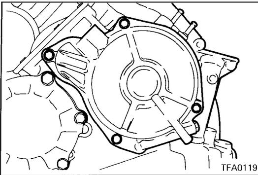
49. Install the end clutch cover and tighten the bolts to the specified torque.
