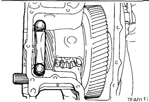
16. Remove the differential cover and gasket.
