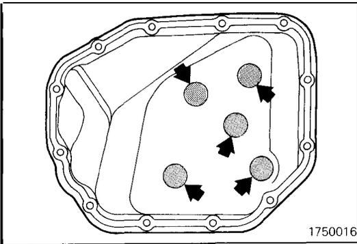
(82) Install five magnets in the five depressions provided inside the oil pan.
