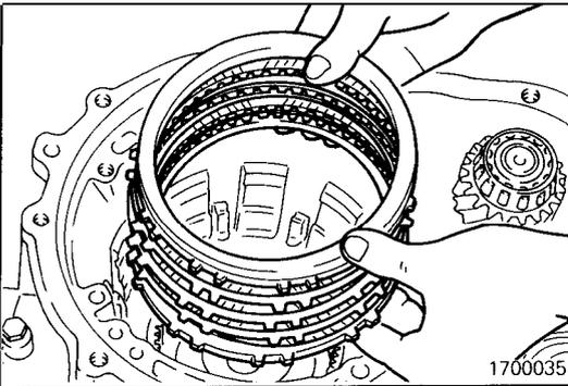
(36) Remove the wave spring, return spring, reaction plate, brake discs, and brake plates.
