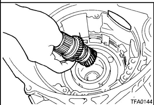
29. Install both sun gears assembled in the previous item into the planetary carrier.
