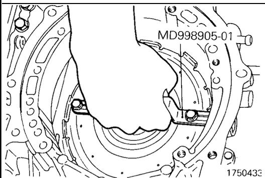
(35) Set the special tool on the center support and remove the center support from the case.
