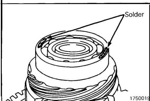
(52) Place approx. 10 mm (.394 in.) long and 2.5 mm (.10 in.) dia. pieces of solder at the locations shown on the differential assembly.
