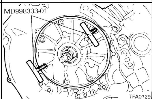
38. Use the special tool to install a new oil pump gasket and oil pump assembly.
