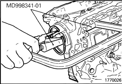
(40) Using the special tools, push in the kickdown servo piston and sleeve assembly, and then install the snap ring.
