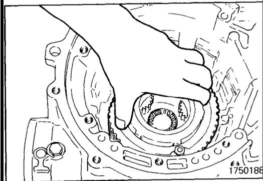
(21) Mount the planetary carrier on the case.
