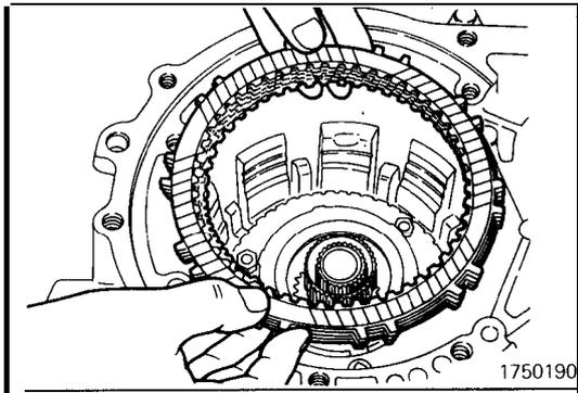
(27) Put the brake disc and brake plate in position.
