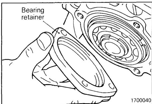
(40) Remove the bearing retainer.
