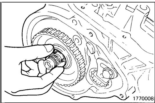
(16) Remove the thrust washer from the input shaft end.
