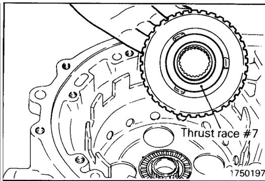
(44) Apply petrolatum jelly to thrust race #7 and attach the thrust race to the rear clutch hub.
