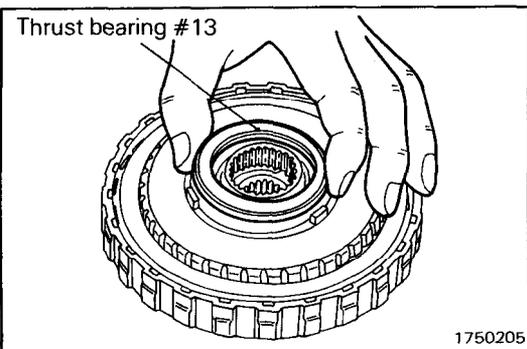
(68) Attach thrust bearing #13 to the end clutch hub with petrolatum jelly.
