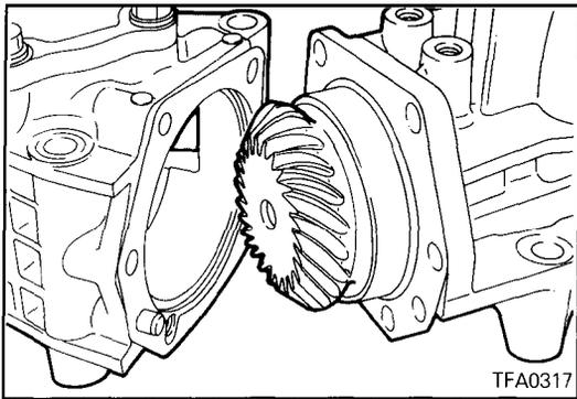
(5) Check to see if the drive bevel gear tooth contact is normal.
