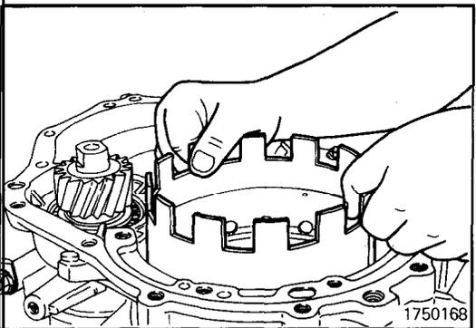
(38) When putting the kickdown drum in the kickdown band, engage the splines of the kickdown drum with those of the reverse sun gear.
