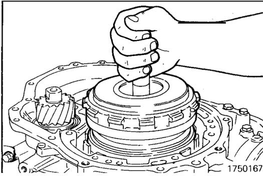
(49) Install the clutch assembly.
