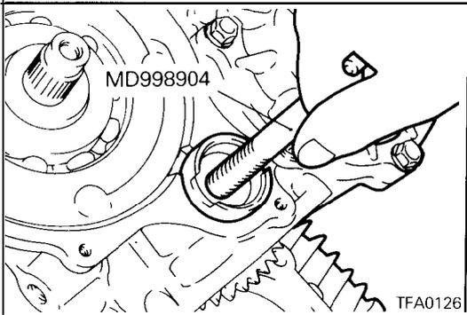
28. Using the special tool, pull out the idler shaft and then remove the idler gear and bearing inner race.
