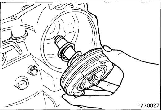
(32) Remove the special tools and then remove the kickdown servo piston, sleeve and spring.
