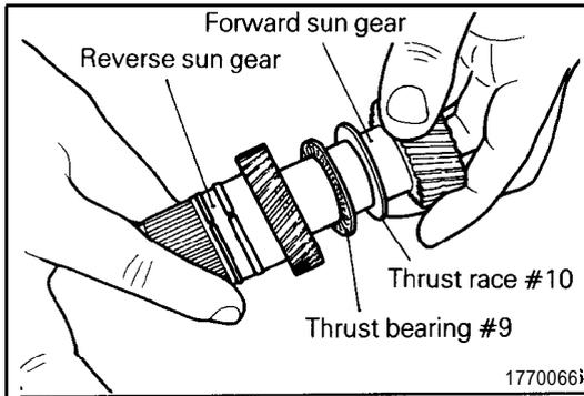
(25) Attach thrust race #10 and thrust bearing #9 to the forward sun gear. Then, assemble the reverse sun gear.
