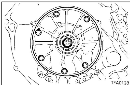
30. Remove oil pump installation bolts.
