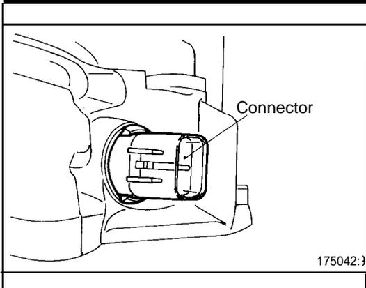
(12) Push catches and remove the solenoid valve connector.
