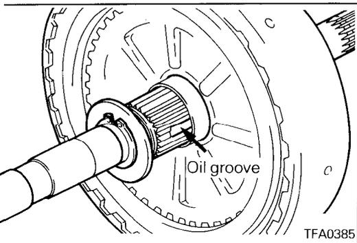
**◆E◆ INPUT SHAFT INSTALLATION**
