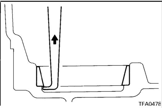
53. Use a sliding hammer, etc., to remove the outer race.
