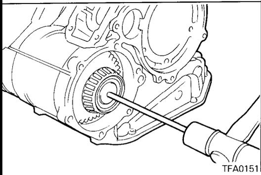
52. Insert a rod 8 mm (.31 in.) in diameter and 200 mm (7.87 in.) in length from the hole shown in the figure and punch out the rear output shaft.
