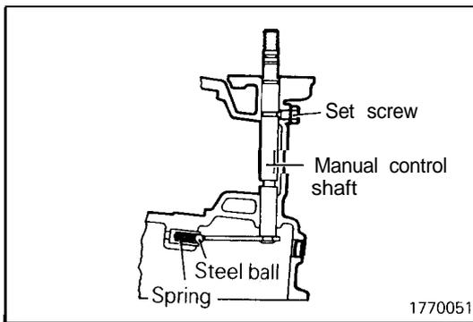
(47) Remove the set screw, and remove the manual control shaft assembly. At this time, remove also the steel ball and spring.
