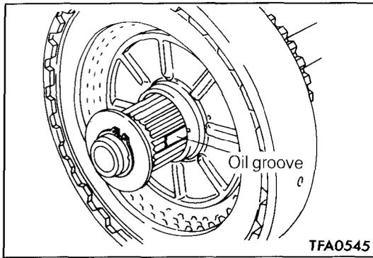
**◆◆ INPUT SHAFT INSTALLATION**
