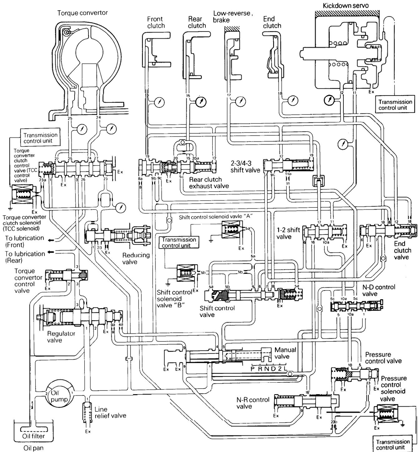
HYDRAULIC CONTROL SYSTEM (Without torque converter clutch)
