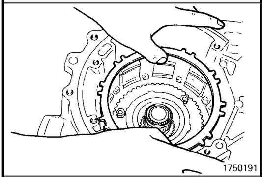
(28) Install the pressure plate which was selected in Step (1).
