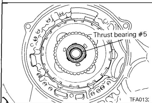
34. Remove the thrust bearing #5.
