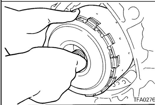
36. Install the clutch assembly and kickdown drum into the transaxle case at the same time.
