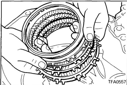
48. Remove the wave spring, return spring, reaction plate, brake discs, and brake plates.
