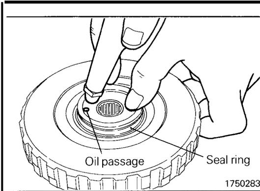
**DISASSEMBLY SERVICE POINT****◆A◆ END CLUTCH PISTON REMOVAL**
