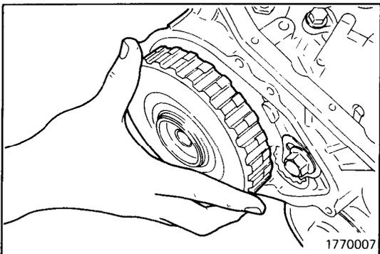
(15) Remove the end clutch assembly.
