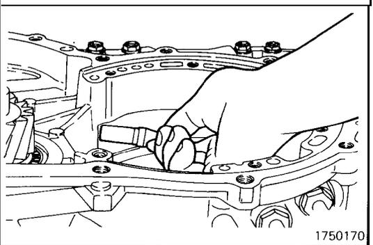
(35) Install the anchor rod, in the transaxle case.
