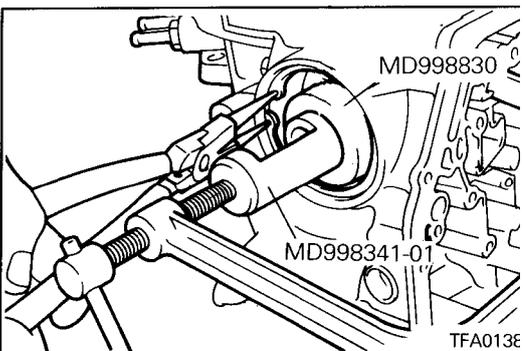
27. Use the special tool to push in the kickdown servo piston and sleeve, and then install a snap ring.
