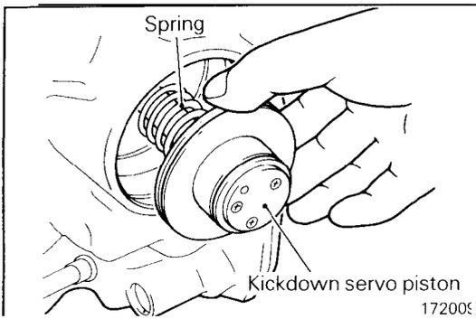
(30) Remove the kickdown servo piston and spring.
