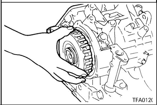
47. Install end clutch assembly.
