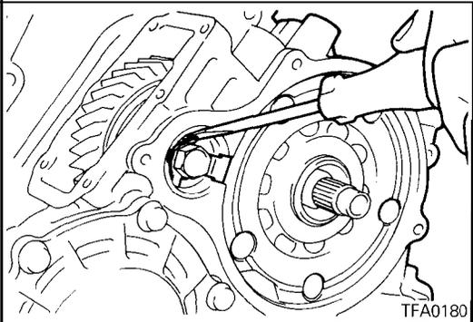
53. Tighten the idler shaft lock bolt together with the new lock plat to the specified torque. Bend the three fingers of the lock plate to prevent turning.
