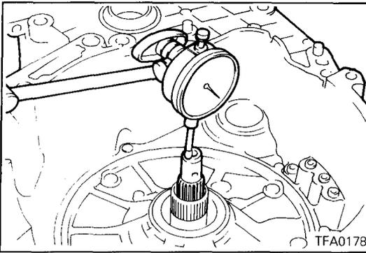
39. Measure the end play of the input shaft. If not the standard value, replace thrust race #3 and thrust washer #1 and adjust to the standard value.
