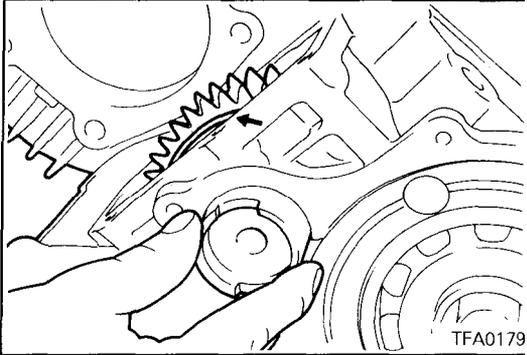
40. Install the spacer, idler gear and bearing and then insert the idler shaft.
