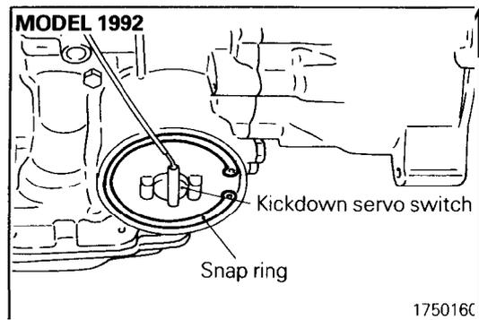
(85) Set a new D-ring in the kickdown servo switch, push the switch into the case and secure it with the snap ring.
