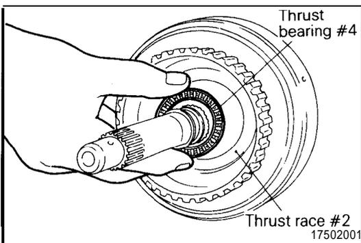
(43) Apply petrolatum jelly to thrust washer #2 and thrust bearing #4 and attach the washer and bearing to the rear clutch assembly.
