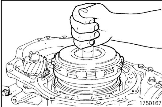
(25) Grasp and raise the input shaft to remove both the front and rear clutch assemblies together.
