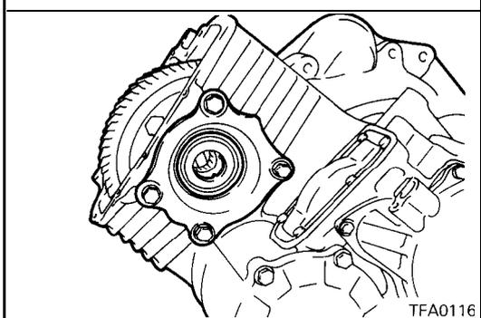
52. Install the differential rear bearing retainer and tighten the bolts to the specified torque.
