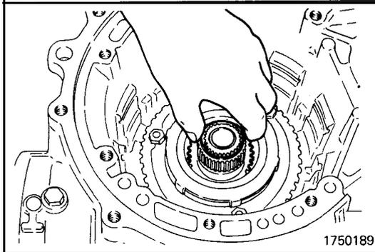
(26) Install the sun gear assembly assembled in step (25) in the planetary carrier.
