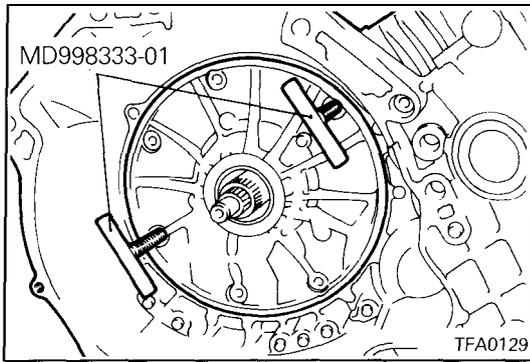
31. Use the special tool and remove the oil pump.
