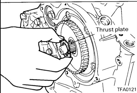
22. Remove the thrust plate.
