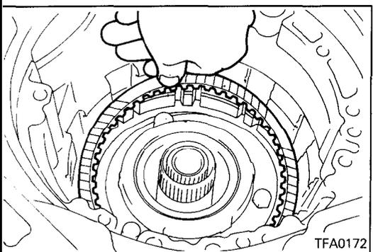
30. Assemble the reaction plate, brake disc and brake plate.
