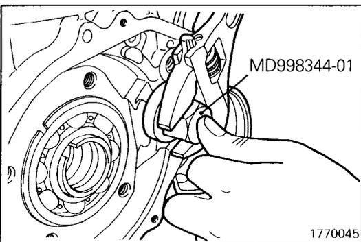
(17) Screw in and tighten the idler shaft by using the special tool.
