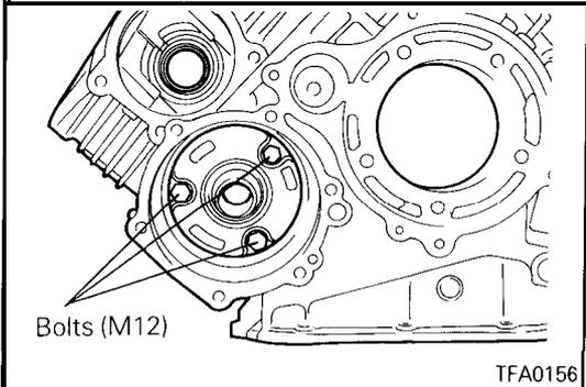
57. Remove the front bearing retainer mounting bolt (M10). Then, screw a bolt (M12) into the threaded hole of the front bearing retainer and, holding that bolt, remove the front bearing retainer and outer race.
