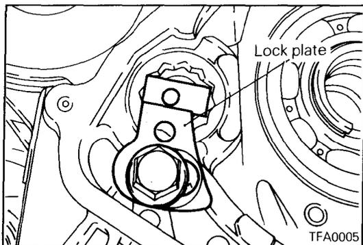
(41) Remove the idler shaft lock plate.
