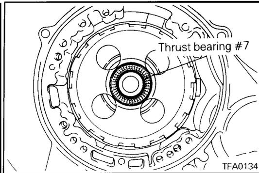
36. Remove the thrust bearing #7
