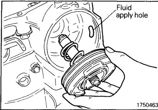
(39) Put the spring on the kickdown servo piston and sleeve assembly, and insert them together in the transaxle case, making sure that the end gap of the teflon seal ring of the kickdown servo piston does not interfere with the fluid apply hole provided in the servo bore of the transaxle case:
