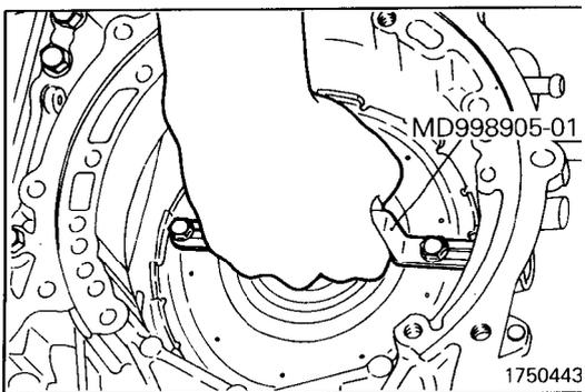
(33) Set the special tool on the center support and remove the center support from the case.
