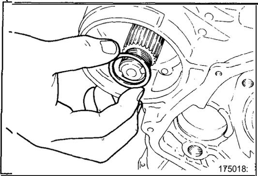
(5) Install the thickest spacer [1.80 mm (.071 in.)].
