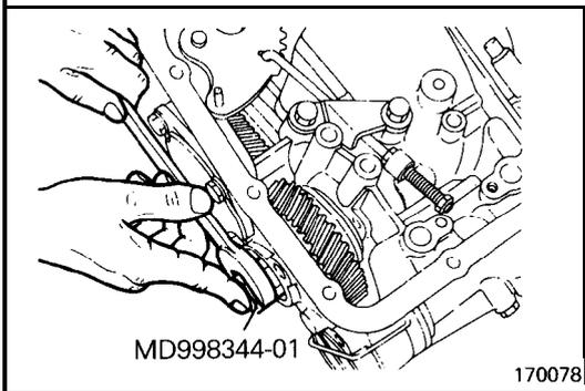
(38) Loosen the transfer idler shaft with the special tool.
