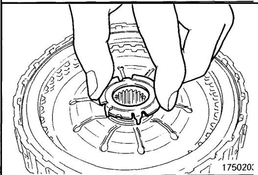
(66) Install the thrust washer on the return spring at the end clutch side.
