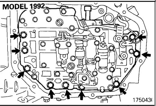
(13) Remove the valve body mounting bolts indicated by arrows and remove the valve body from the transaxle case.
