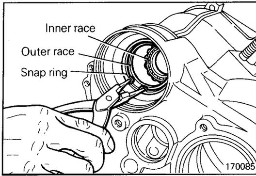
(45) Remove the snap ring, and then the tapered roller bearing inner and outer races.
