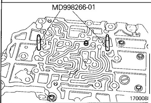
**G** LOWER VALVE BODY SUB ASSEMBLY INSTALLATION
