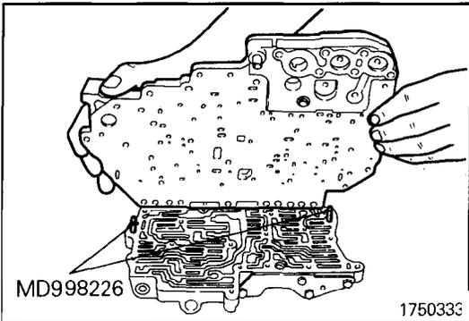
**▶B▶ UPPER VALVE BODY SUB ASSEMBLY INSTALLATION**
