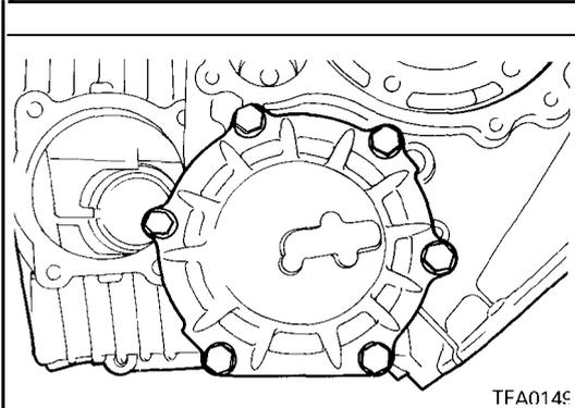
17. Install the output bearing retainer and tighten the bolts to the specified torque.
