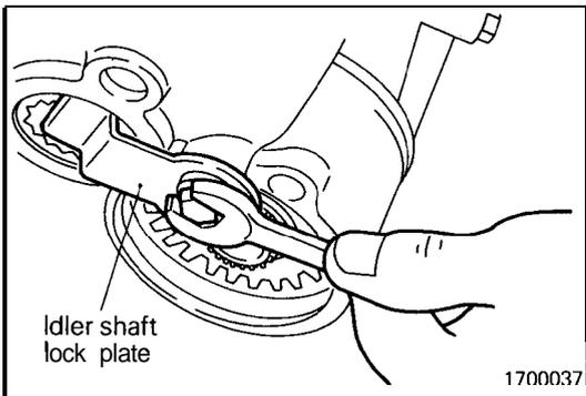
(37) Remove the idler shaft lock plate.
