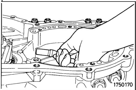
(32) Install the anchor rod, in the transaxle case.
