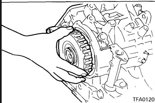
59. Install end clutch assembly.
