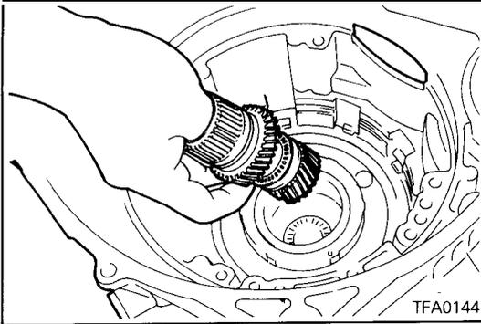
46. Remove reverse sun gear and forward sun gear together.
