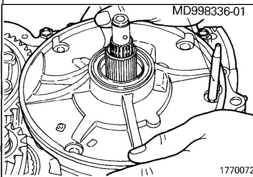
(48) Attach the special tool to the transaxle case. Using the tool as a guide, first install a new oil pump gasket and then the oil pump in the case.
