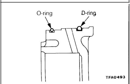
(35) Install a new O-ring and D-ring on the kickdown servo sleeve, and apply a very thin coat of automatic transaxle fluid to the rings.
