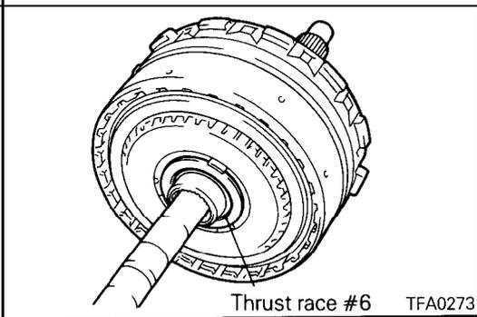
33. Install thrust race #6 on the end of the rear clutch hub.
