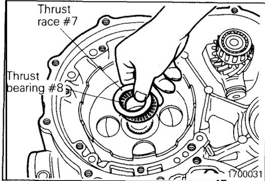
(25) Remove thrust race #7 and thrust bearing #8.
