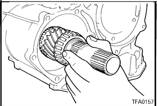
58. Remove the front output shaft.
