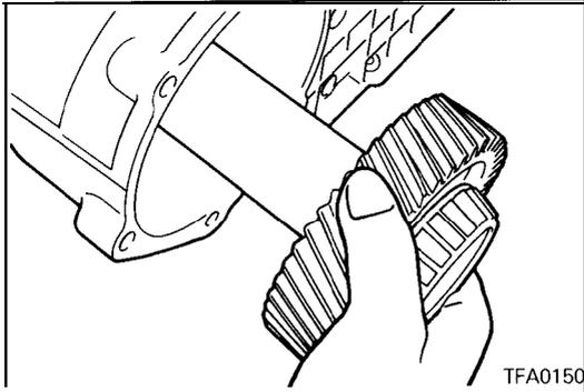
52. Remove the transfer shaft.
