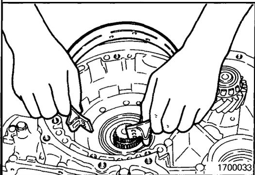
(37) Install the kickdown band; attach the ends of the band to the ends of the anchor rod and servo piston rod.
