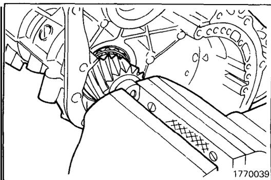
(7) Remove the special tool and secure the transfer shaft in position.
