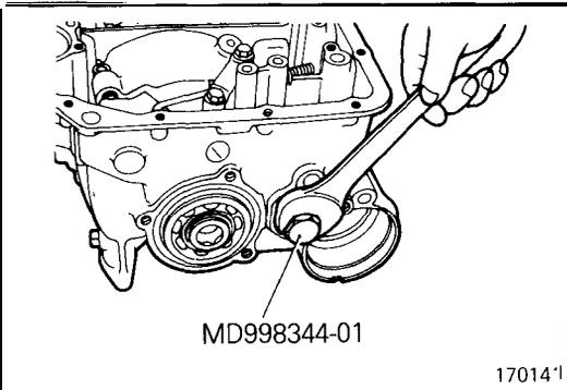
(9) Screw in and tighten the idler shaft by using the special tool.
