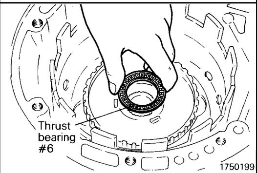
(46) Apply petrolatum jelly to thrust bearing #6 and attach it to the clutch hub.
