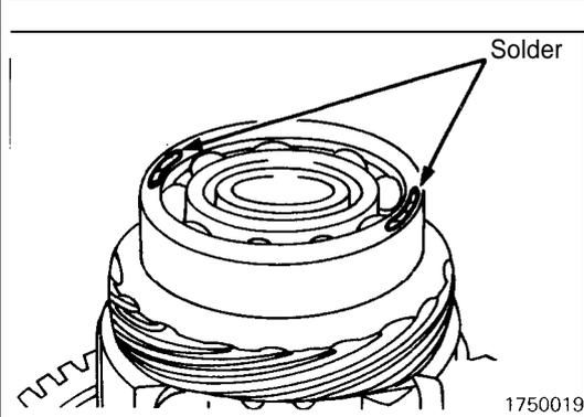
(56) Place approx. 10 mm (.394 in.) long and 2.5 mm (.10 in.) dia. pieces of solder at the locations shown on the differential assembly.
