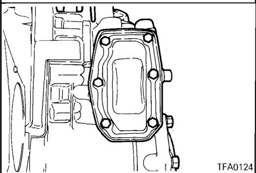
54. Install the idler gear cover and a new gasket.
