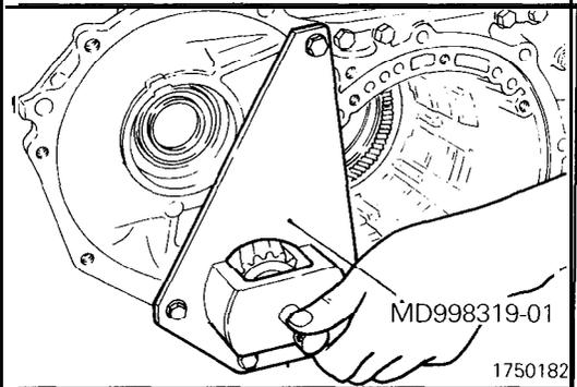
(4) Mount the special tool on the transaxle case to support the transfer shaft.
