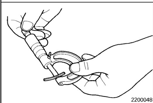
19. Remove the outer race from the output bearing retainer and remove the solder. If the solder is not crushed, repeat steps (4) – (6), using the solder with diameter of 3 mm (.12 in.). Measure the thickness of the crushed solder with a micrometer and select a spacer with a thickness that will provide the standard value for the preload.
