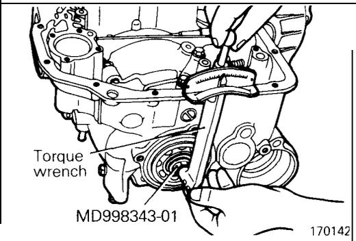
(10) Insert the special tool into the output flange and measure the preload using a low reading torque wrench. Adjust the preload to the standard value by tightening or loosening the transfer idler shaft.
