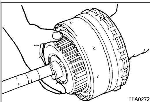
44. Install the rear clutch hub on the rear clutch.
