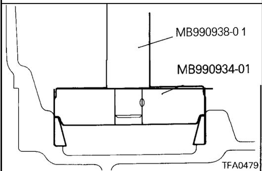
2. Use the special tool to press fit the outer race into the transaxle case.
