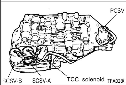
**SOLENOID VALVE ASSEMBLY INSTALLATION**
