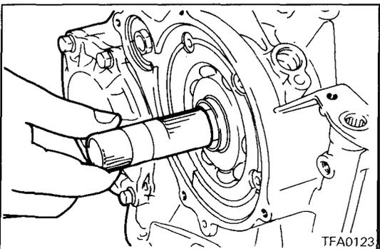
43. Insert the end clutch shaft from the end with the long spline.
