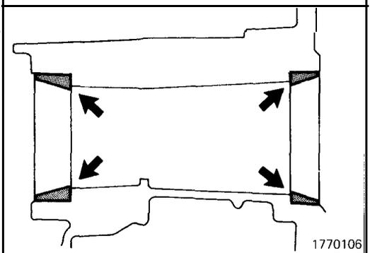
(52)Remove the outer races from the transfer shaft bearing.
