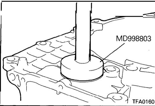
2. Using the special tool, install the rear output shaft oil seal.
