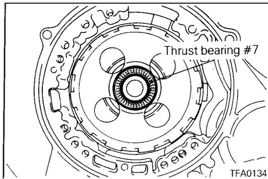
36. Remove the thrust bearing #7.
