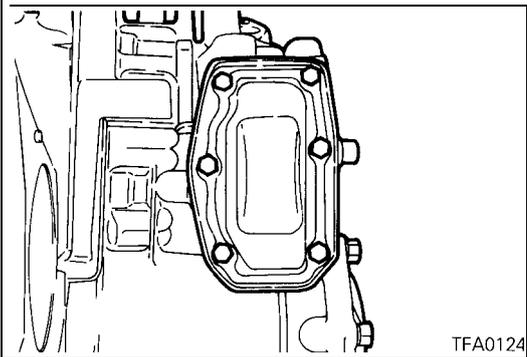
26. Remove the idler gear cover mounting bolts, then remove the idler gear cover and gasket.
