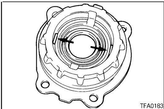
51. Place solder with a length of approximately 10 mm (.39 in.) and diameter of 1.6 mm (.06 in.) on the differential rear bearing retainer at the position shown in the diagram and install the outer race.
