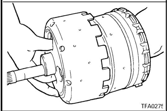
47. Install the clutch assembly in the kickdown drum.
