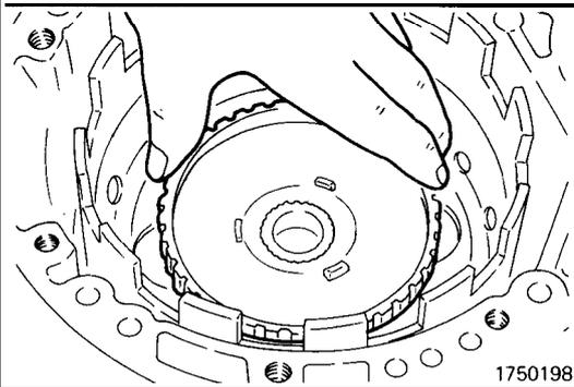
(45) Install clutch hub, engaging it with the forward sun gear splines.
