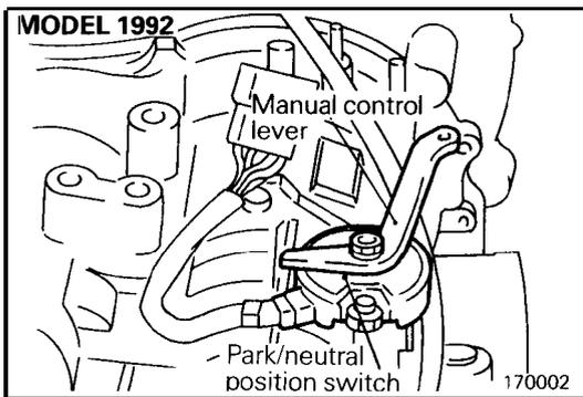
(8) Remove the manual control lever, and then remove the park/neutral position switch (PNP switch).
