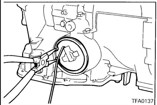
39. Remove the kickdown servo cover snap ring. Then remove the kickdown servo switch.
