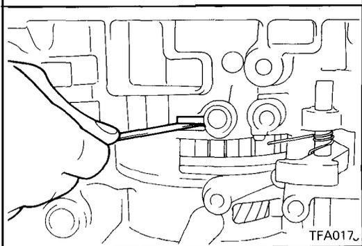
23. Use a thickness gauge and measure the end play of the low/reverse brake. Adjust to the standard value by selecting the proper pressure plate.
