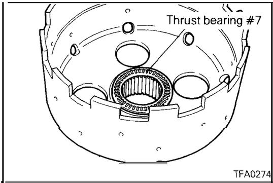
46. Install thrust bearing #7 in the kickdown drum.
