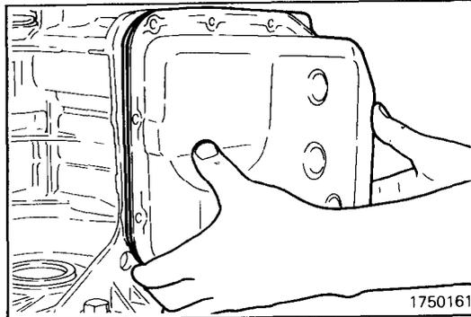
(8) Remove the oil pan and oil pan gasket.
