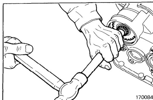
(44) Drive the transfer shaft out toward the torque converter housing to remove the shaft and the transfer driven gear.
