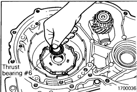
(42) Apply petrolatum jelly to thrust bearing #6 and attach it to the clutch hub.
