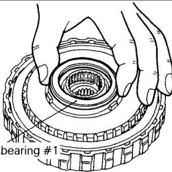
58. Adhere thrust bearing #1 to the end of the clutch hub with petrolatum.
