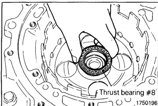
(43) Apply petrolatum jelly to thrust bearing #8 and attach the thrust bearing to the kickdown drum.
