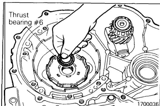
(23) Remove thrust bearing #6.
