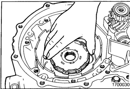
(41) Install the rear clutch hub, engaging it with the forward sun gear splines.
