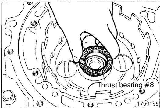
(39) Apply petrolatum jelly to thrust bearing #8 and attach the thrust bearing to the kickdown drum.
