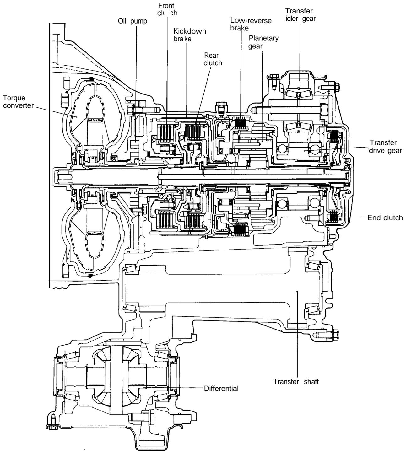
SECTIONAL VIEW – W4A32 with torque converter clutch
