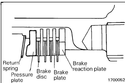
(b) Install the pressure plate and mount the return spring.
