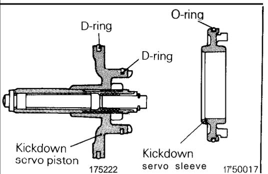
(36) Install a new teflon seal ring and a new D-ring in the grooves of the kickdown servo piston, and apply automatic transaxle fluid to the rings.
