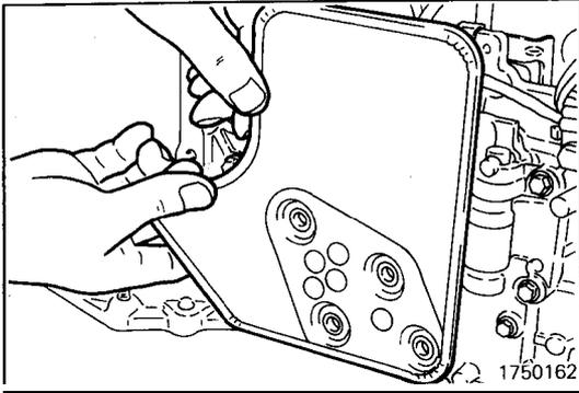
(74) Install the oil filter and tighten the four oil filter mounting bolts to the specified torque.
