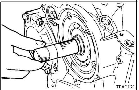
25. Pull out the end clutch shaft.
