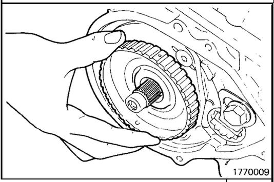
(17) Remove the end clutch hub and the thrust bearing.
