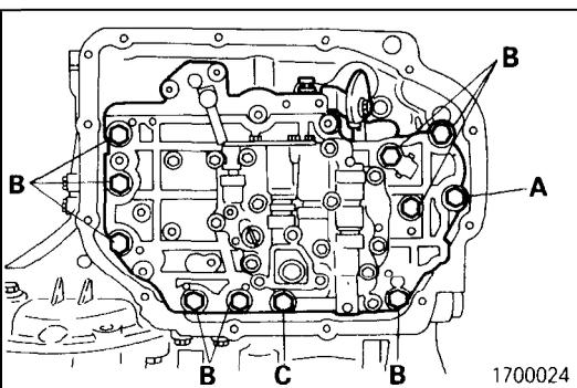
(73) Tighten the valve body mounting bolts (10 pieces) to the specified torque.
