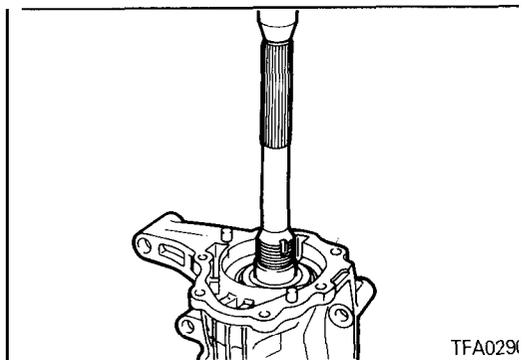
**◁B▷ DRIVEN BEVEL GEAR ASSEMBLY REMOVAL**
