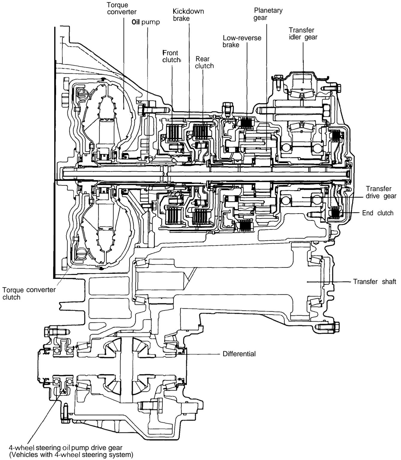
SECTIONAL VIEW – F4A33 without torque converter clutch
