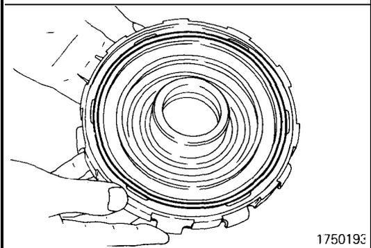
32. Apply a coating of petrolatum jelly to the wave spring and attach it to the center support.
