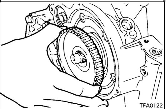
23. Remove the end clutch hub.
