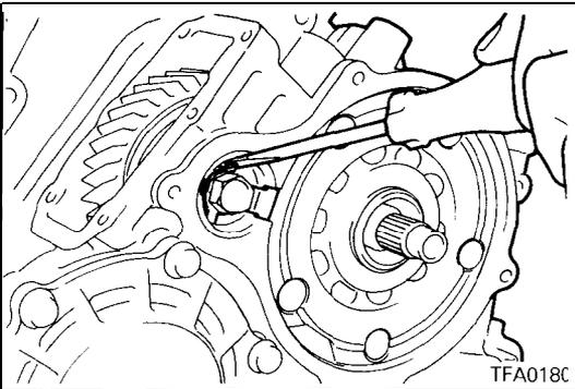
41. Tighten the idler shaft lock bolt together with the new lock plat to the specified torque. Bend the three fingers of the lock plate to prevent turning.
