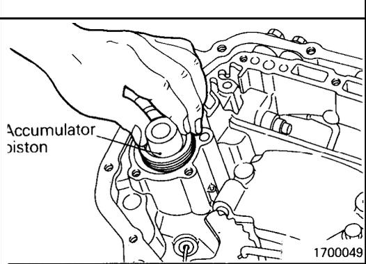
(15) Remove the two accumulator springs, then remove the accumulator piston from the transaxle case.
