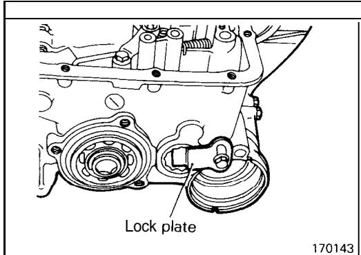
(11) After completing the preload adjustment, install the idler shaft lock plate. The clearance between the idler shaft and the lock plate should be closed in the direction that will prevent idler shaft looseness, and then tighten the lock plate bolt to specified torque.
