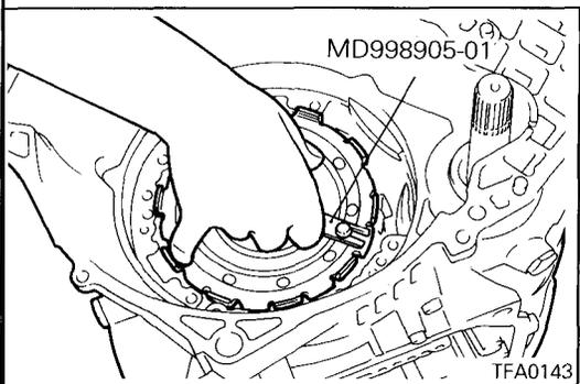
45. Using the special tool, remove the center support.
