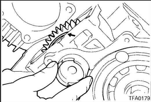
52. Install the spacer, idler gear and bearing and then insert the idler shaft.
