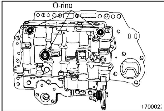
(67) Install the O-rings in the O-ring grooves at three locations on the valve body.
