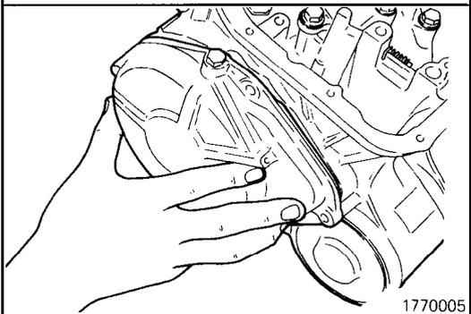
(71) Secure the end clutch cover by tightening its mounting bolts to specified torque.
