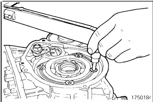
(20) Install the bearing retainer.
