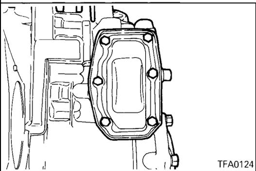
42. Install the idler gear cover and a new gasket.
