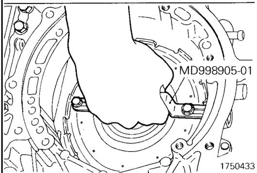
(32) Attach the special tool to the center support. Install the center support slowly in the transaxle case, grasping the special tool.
