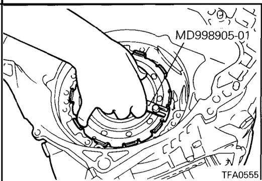
21. Mount the special tool on the center support, install 2 new O-rings and push into the transaxle case.
