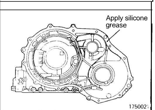
(62) Apply silicone grease to all gasket surfaces of the transaxle case.
