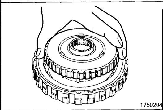
(67) Install the end clutch hub on the end clutch assembly.
