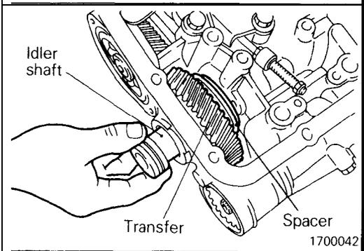
(8) Place the transfer idler gear in the case, and insert and screw the idler shaft into position.
