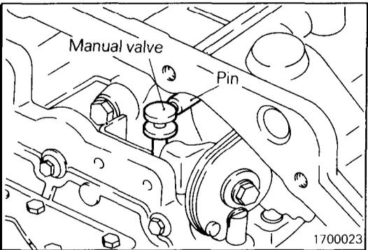
(70) Install the valve body in the transaxle case while fitting the detent plate pin in the gap between the lands of the manual valve.
