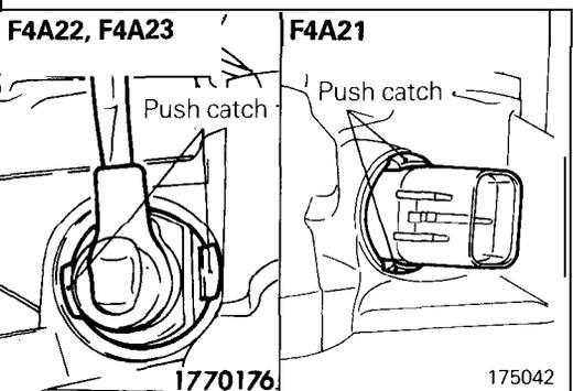
(12) With their catches pressed down, force the harness grommet and connector into the transaxle case.
