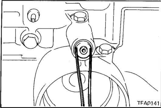
36. Install the air exhaust plug, and then install the plug.
