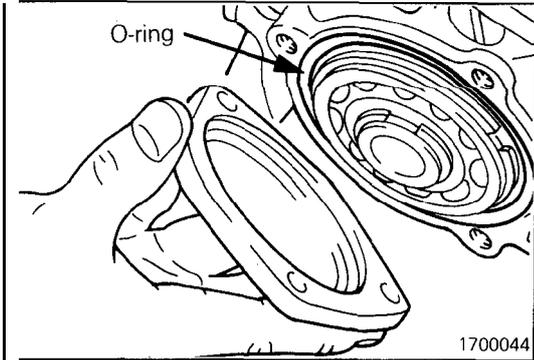
(12) Install a new O-ring in the groove of the transaxle case, and then install the bearing retainer.
