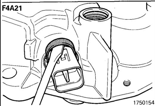
(11) Remove the clip from the solenoid valve connector (F4A21 only).
