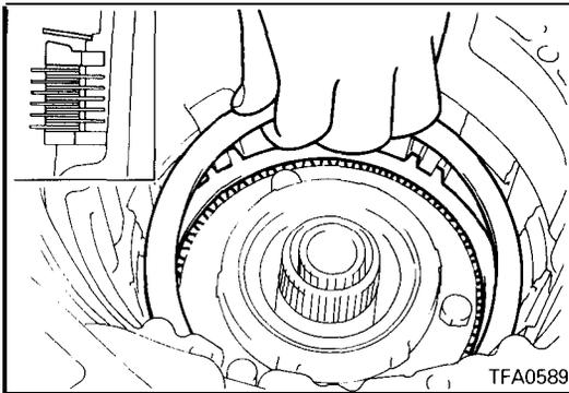
19. Assemble the pressure plate used in disassembly and install the return spring.
