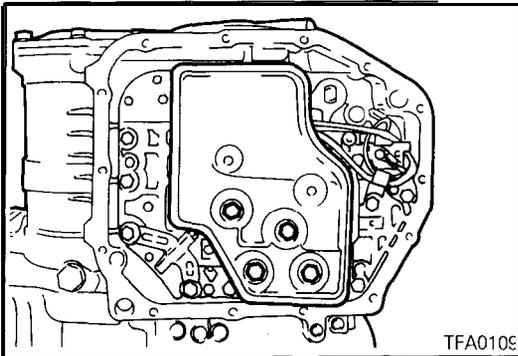
8. Remove the oil filter from the valve body.
