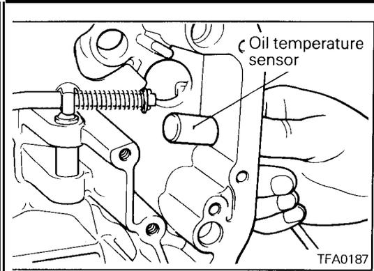
74. Insert the oil temperature sensor into the case.
