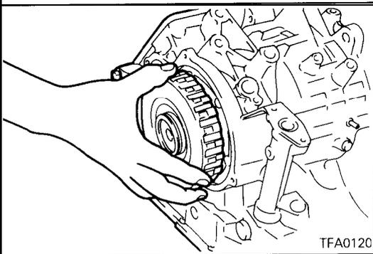
21. Remove the end clutch assembly.
