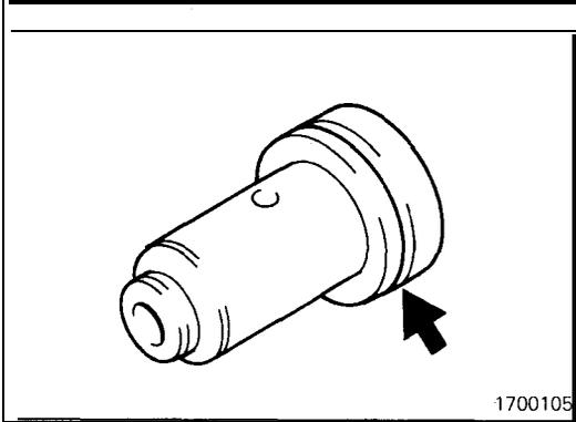
(7) Install a new O-ring in the groove of the idler shaft, and apply a very thin coat of automatic transmission fluid to the O-ring.
