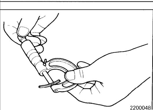
(60) Measure the thickness of the flattened solder using a micrometer. Add the measured solder thickness (T) to the value 0.38 mm (.015 in.), which corresponds to the gasket thickness.
