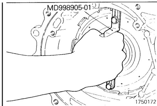
(29) Attach the special tool to the center support and install the support in the transaxle case.
