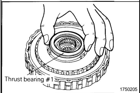
46. Adhere thrust bearing #1 to the end of the clutch hub with petrolatum.
