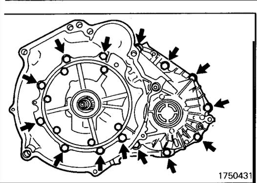
(16) Remove the 14 bolts indicated by arrows and remove the converter housing and gasket.
