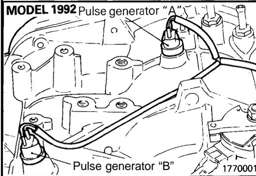
(89) Install pulse generators "A" and "B" and tighten the bolt to the specified torque.
