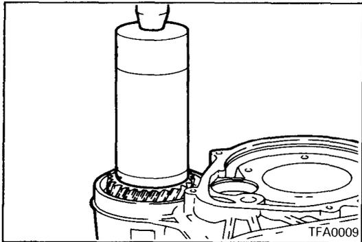
(6) Install the transfer driven gear on the transfer shaft
