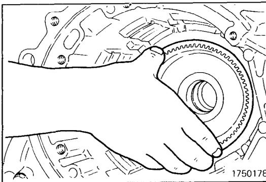
(46) Remove the output flange from the case.
