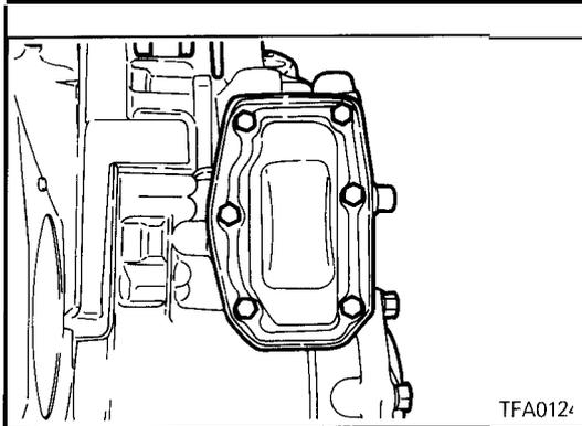
26. Remove the idler gear cover mounting bolts, then remove the idler gear cover and gasket.
