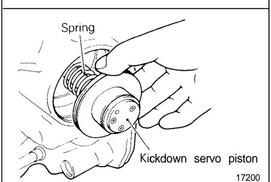
(33) Install new seal rings in the grooves of the kickdown servo piston and coat the rings with automatic transaxle fluid.
