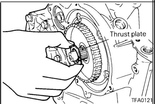
22. Remove the thrust plate.
