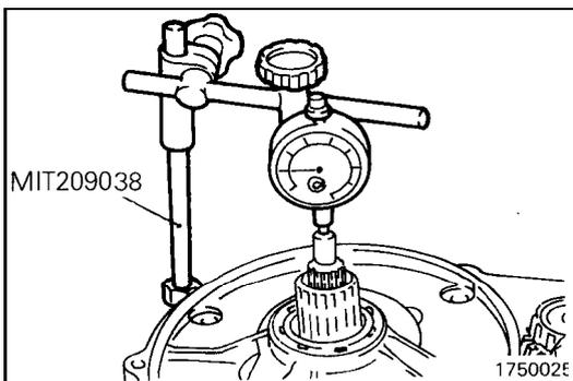
(55) Measure the end play of the input shaft. If the measurement is out of specification, replace thrust race #3 and thrust washer #1 to meet the specification.
