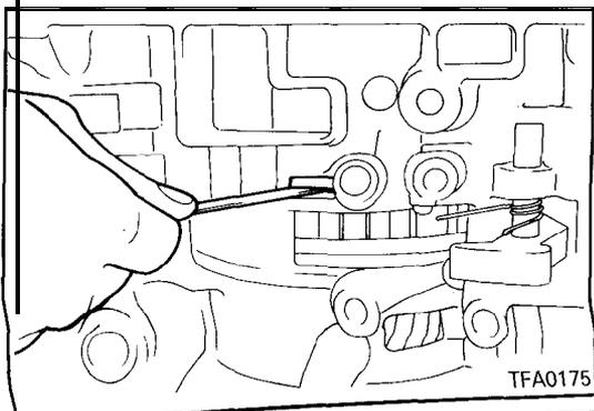
35. Use a thickness gauge and measure the end play of the low/reverse brake. Adjust to the standard value by selecting the proper pressure plate.
