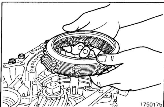
(38) Remove the wave spring, return spring, reaction plate, brake discs, and brake plates.
