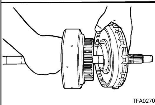
30. Combine the rear clutch assembly and the front clutch assembly.
