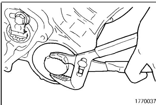
(47) Remove the transfer shaft cover.
