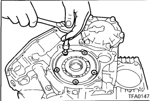
12. Install the bearing retainer using new bolts.
