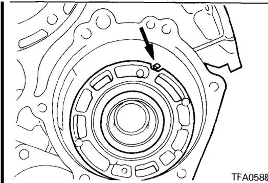
14. Install the center bearing retainer so the projection of the stopper bolt fits in the groove of the center bearing retainer.
