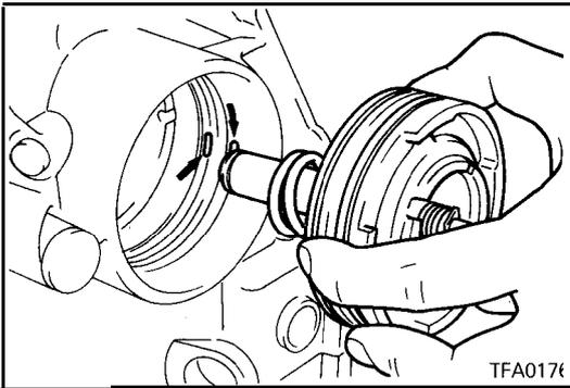
26. Install the kickdown servo spring, piston and sleeve.
