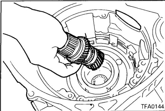
17. Install both sun gears assembled in the previous item into the planetary carrier.
