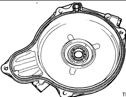
60. Attach a new O-ring to the end clutch cover.
