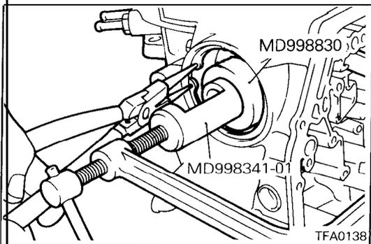
40. Using the special tool, push in the kickdown servo and remove the snap ring.
