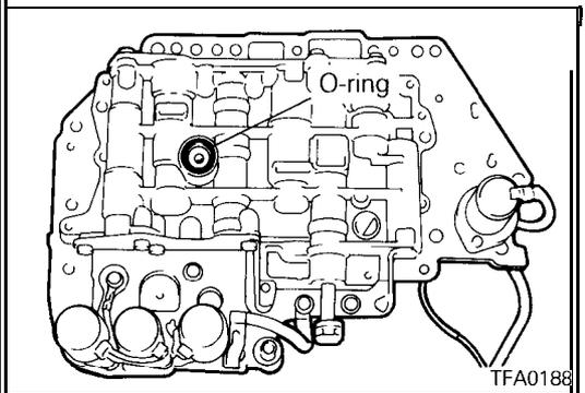
75. Install an O-ring in the O-ring groove at the top of the valve body assembly.
