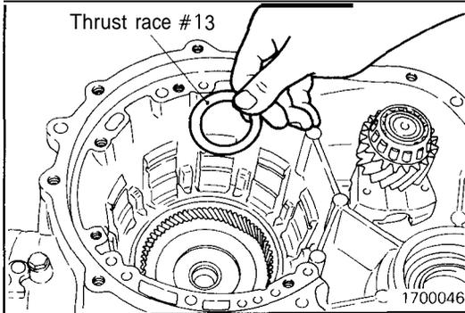
(19) Coat thrust race #13 with petrolatum jelly and attach it to the output flange.
