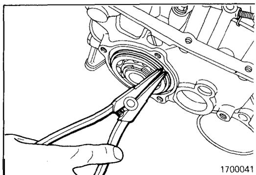
(41) Remove the snap ring from the output flange bearing.
