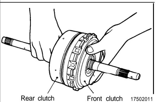
(48) Mate the rear clutch assembly with the front clutch assembly.
