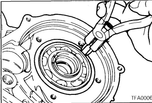
(45) Remove the snap ring from the output flange bearing.
