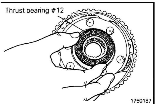
(23) Apply petrolatum jelly to thrust bearing #12 and secure the bearing on the planetary carrier.
