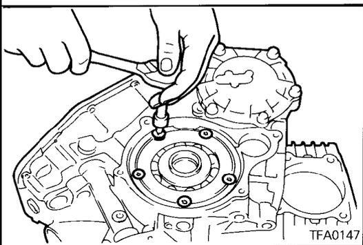
49. Remove the screws and the rear bearing retainer.
