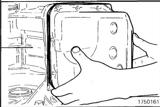
(83) Clean the gasket surfaces of the transaxle case and oil pan. Install a new oil pan gasket and then the oil pan by tightening the 12 bolts to the specified torque.
