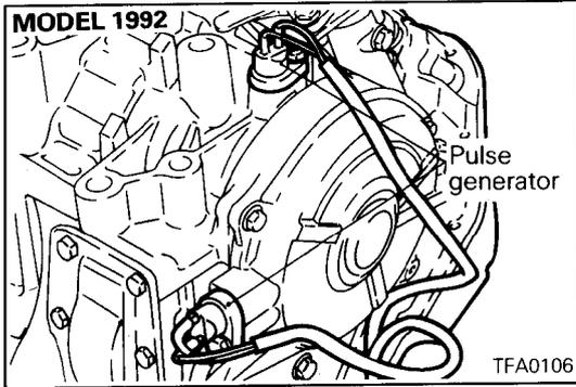
5. Remove the pulse generator "A" and "B"
