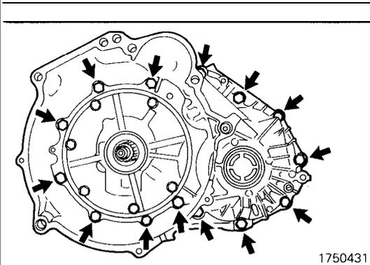
(57) Install the converter housing directly to the transmission case without installing the rubber coated metal gasket.
