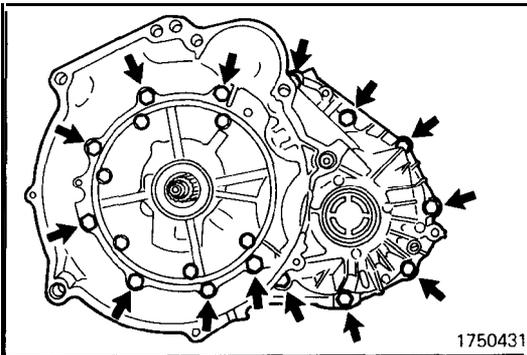
(63) Install a new gasket on the transaxle case.
