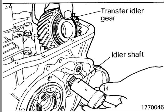
(16) Place the transfer idler gear in the case, and insert and screw the idler shaft into position.
