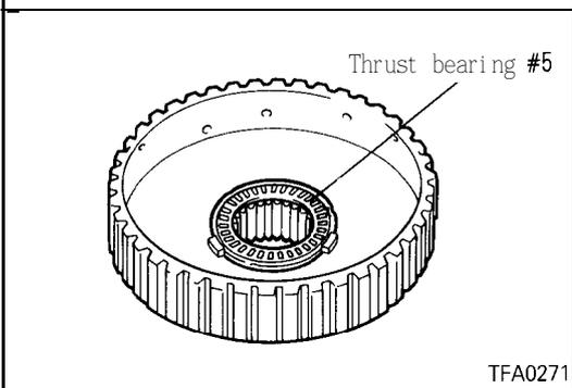
31. Install thrust bearing #5 on the rear clutch hub.
