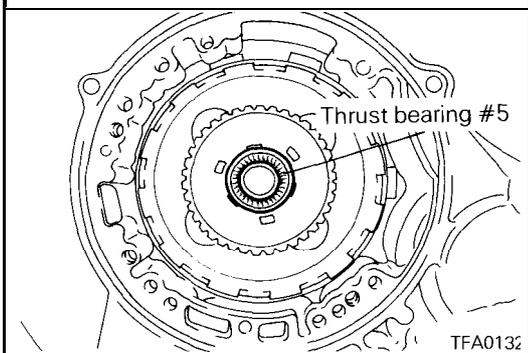
34. Remove the thrust bearing #5
