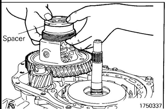
(23) Remove the spacer and differential from the transaxle case.
