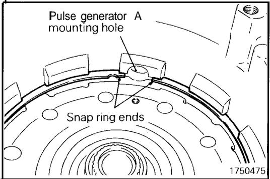
(34) Install the snap ring to secure the center support. The snap ring ends should not interfere with the pulse generator mounting hole.
