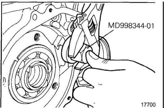
(42) Loosen the transfer idler shaft with the special tool.
