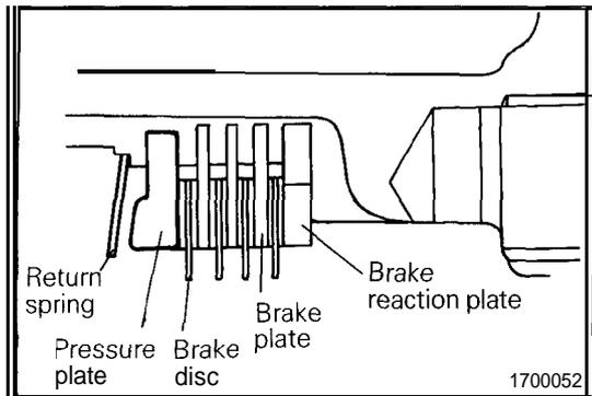
(25) Install the brake pressure plate which was selected in Step (1).
