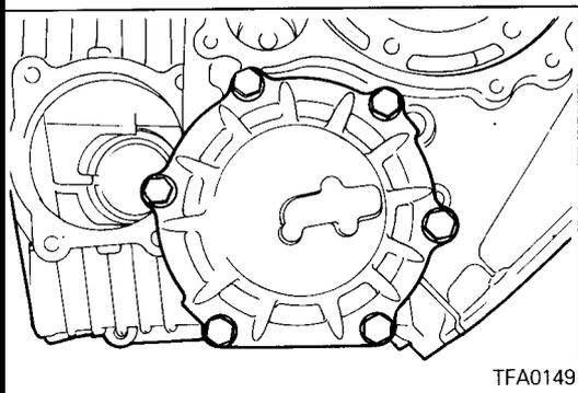
51. Remove the output bearing retainer mounting bolts and then remove the output bearing retainer and outer race.
