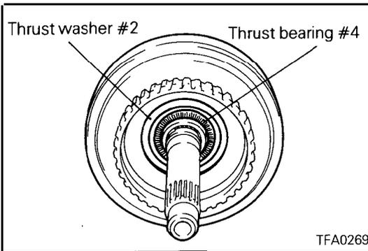
29. Install thrust bearing #4 and thrust washer #2 on the rear clutch.
