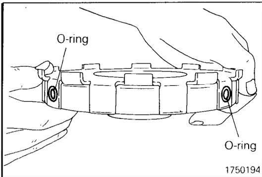
(31) Install the two new O-rings on the hydraulic pressure holes of the center support.
