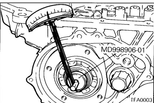
(18) Insert the special tool into the output flange and measure the preload using a low reading torque wrench. Adjust the preload to the standard value by tightening or loosening the transfer idler shaft.
