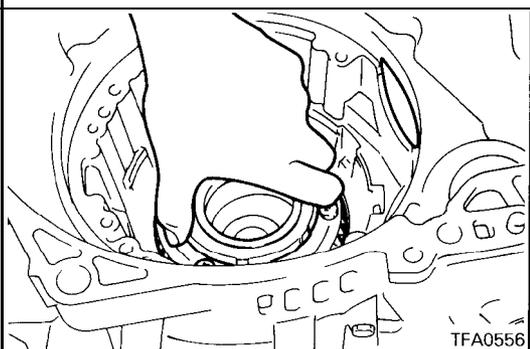
15. Assemble the planetary carrier.
