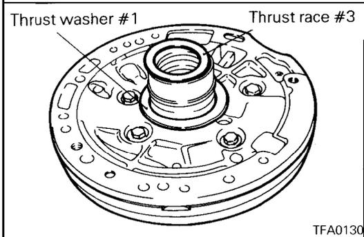
37. Adhere thrust race #3 and thrust washer #1 to the back of the oil pump with petrolatum.
