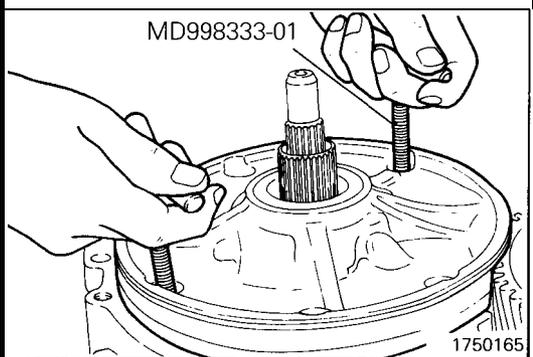
(22) Grasping the special tools, remove the oil pump. Then, remove the gasket.
