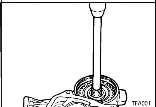
(51)Drive out the transfer shaft toward the converter housing end and remove the transfer shaft and transfer driven gear.
