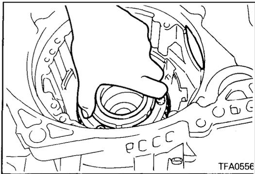
27. Assemble the planetary carrier.
