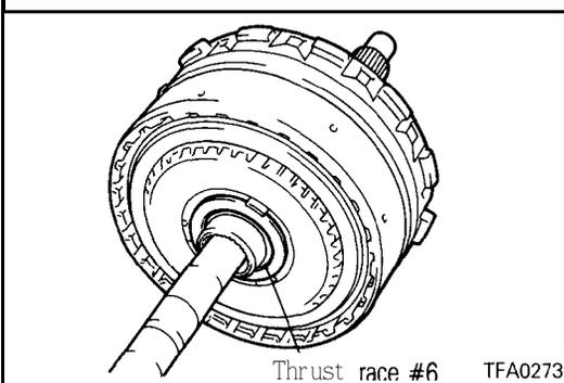
45. Install thrust race #6 on the end of the rear clutch hub.
