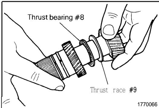
28. Assemble the forward sun gear, thrust race #9, thrust bearing #8 and reverse sun gear.
