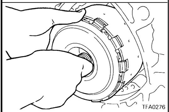
48. Install the clutch assembly and kickdown drum into the transaxle case at the same time.
