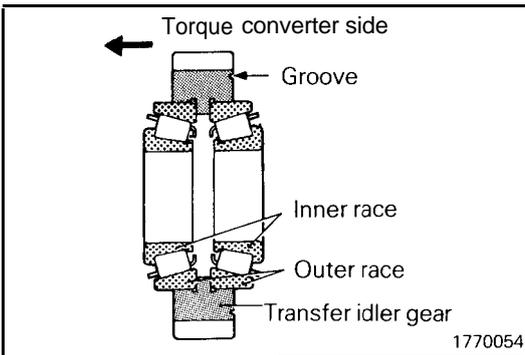
(15) Install the bearing outer race and inner races in the transfer idler gear.
