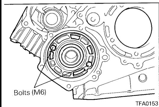
54. Put a bolt (M6) into the center bearing retainer and, holding that bolt, remove the center bearing retainer and outer race.
