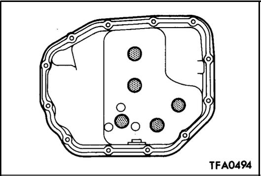
(75) Install the magnet to one of the recesses provided inside the oil pan.
