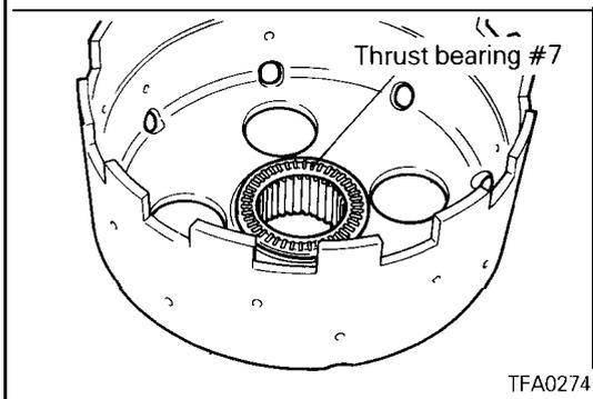
34. Install thrust bearing #7 in the kickdown drum.
