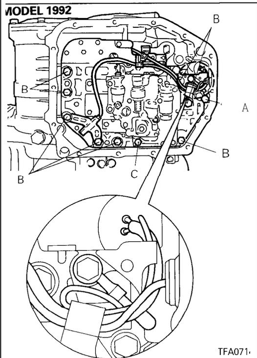
67. Insert the knock pin of the valve body into the case, keeping the detent plate pin in the manual valve groove. Temporarily install the valve body, install the oil temperature sensor and holder; then tighten the mounting bolts to the specified torque.
