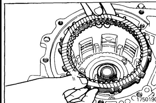
(24) Put the brake disc and brake plate in position.
