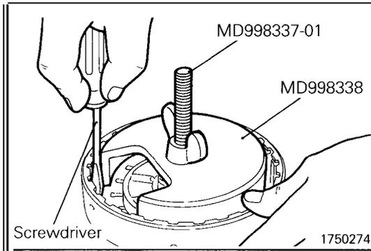
**DISASSEMBLY SERVICE POINTS****◀A▶ WAVE SPRING REMOVAL**
