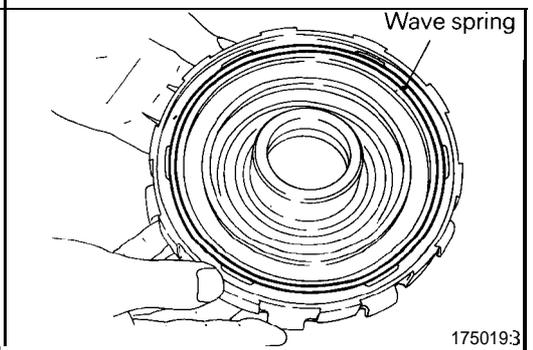
(30) Apply petrolatum jelly to the wave spring and attach the wave spring to the center support.
