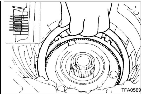
31. Assemble the pressure plate used in disassembly and install the return spring.
