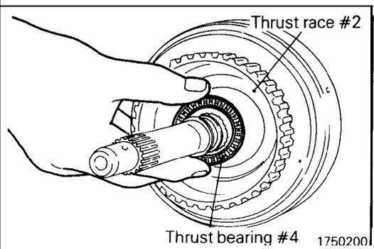
(47) Apply petrolatum jelly to thrust washer #2 and thrust bearing #4 and attach the washer and bearing to the rear clutch assembly.
