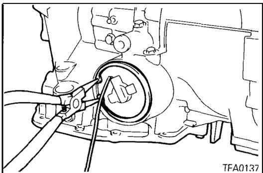
77. Install the kickdown servo switch and fasten with a snap ring.
