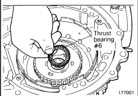
(26) Remove thrust bearing #6.
