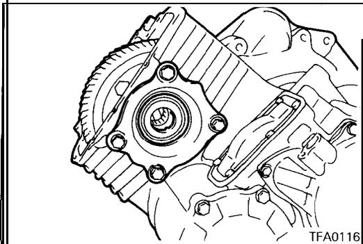
18. Remove the differential bearing retainer, spacer and outer race.
