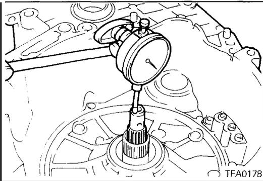
51. Measure the end play of the input shaft. If not the standard value, replace thrust race #3 and thrust washer #1 and adjust to the standard value.
