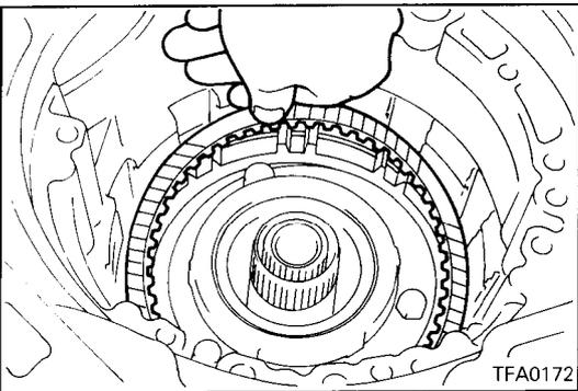
18. Assemble the reaction plate, brake disc and brake plate.
