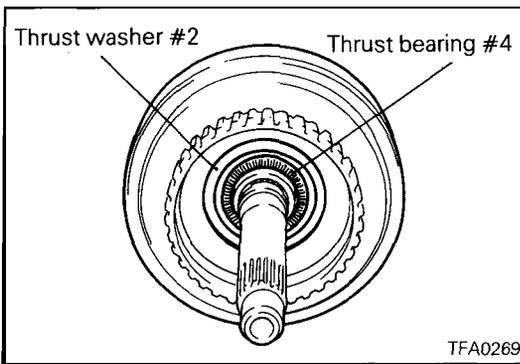
41. Install thrust bearing #4 and thrust washer #2 on the rear clutch.
