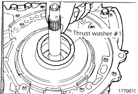
(21) Remove fiber thrust washer #1.
