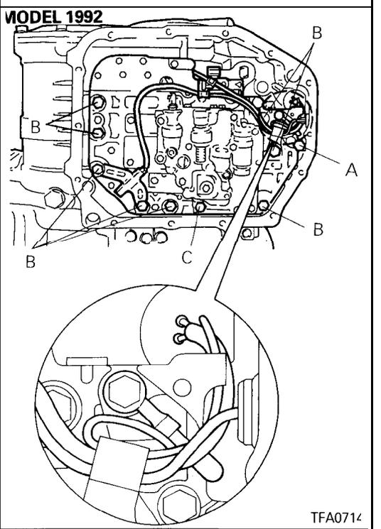
79. Insert the knock pin of the valve body into the case, keeping the detent plate pin in the manual valve groove. Temporarily install the valve body, install the oil temperature sensor and holder; then tighten the mounting bolts to the specified torque.
