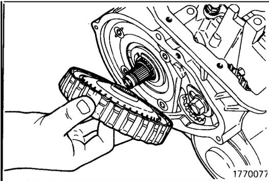
(69) Install the end clutch assembly.
