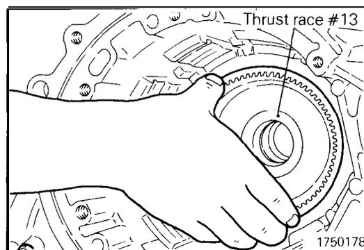
(42) Remove the output flange and thrust race #13 from the case.
