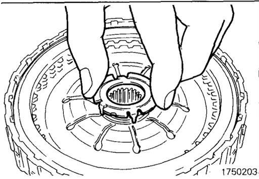
56. Fit the thrust washer on the return spring of the end clutch.
