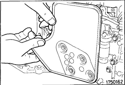
(81) Install the oil filter and tighten the four oil filter mounting bolts to the specified torque.
