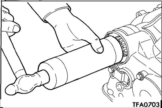
(15) Use the special tool to install the bearing inner race on the transfer shaft.
