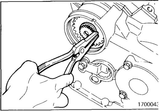
(18) Install the snap ring on the end of the transfer shaft.
