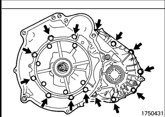
(19) Remove the 14 bolts indicated by arrows and remove the converter housing and gasket.
