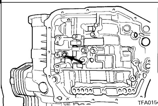
55. Remove the center bearing retainer stopper bolt.
