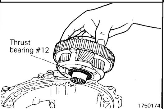
(37) Remove the planetary gear set and thrust bearing #12.
