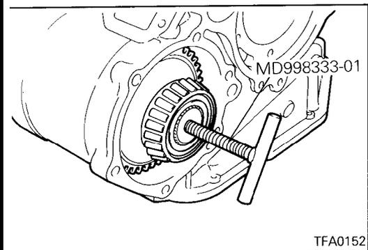
53. Using the special tool, remove the center differential.
