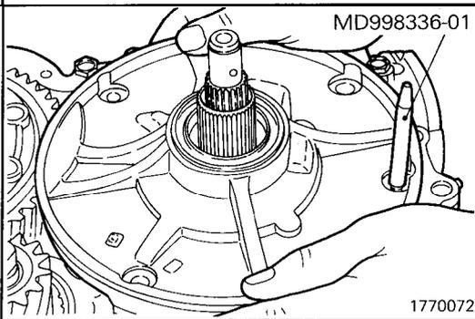
(52) Install the special tool on the transaxle case. Using the special tool as a guide, install a new oil pump gasket and the oil pump in the case.
