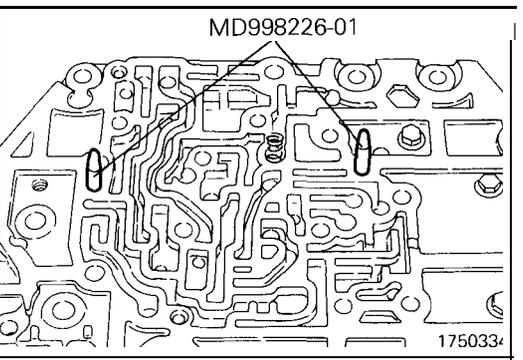
**▶D▶ LOWER VALVE BODY SUB ASSEMBLY INSTALLATION**
