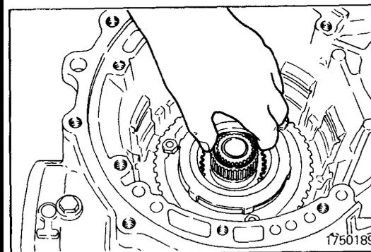
(23) Install the sun gear assembly assembled in step (22) in the planetary carrier.
