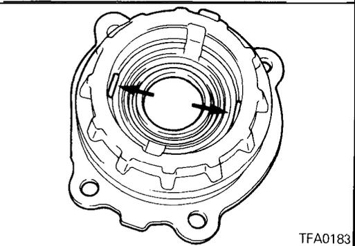
63. Place solder with a length of approximately 10 mm (.39 in.) and diameter of 1.6 mm (.06 in.) on the differential rear bearing retainer at the position shown in the diagram and install the outer race.
