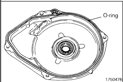
(70) Install new O-ring in the groove of the end clutch cover. Check the bearing for smooth rotation and replace it if defects are evident. Apply an ample amount of automatic transmission fluid to the bearing.
