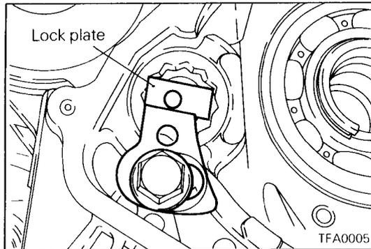
(19) After completing the preload adjustment, install the idler shaft lock plate. The clearance between the idler shaft and the lock plate should be closed in the direction that will prevent idler shaft looseness, and then tighten the lock plate bolt to the specified torque.
