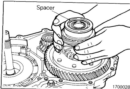
(20) Remove the spacer and differential from the transaxle case.
