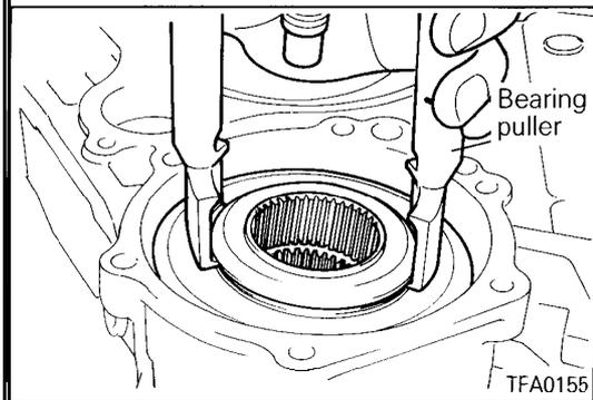
56. First remove the stopper ring and then put a bearing puller or similar tool in the viscous coupling groove and pull out the viscous coupling.
