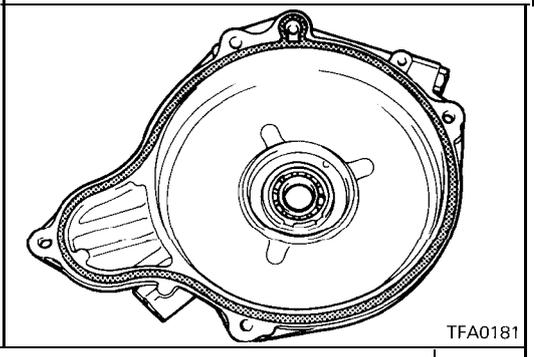
48. Attach a new O-ring to the end clutch cover
