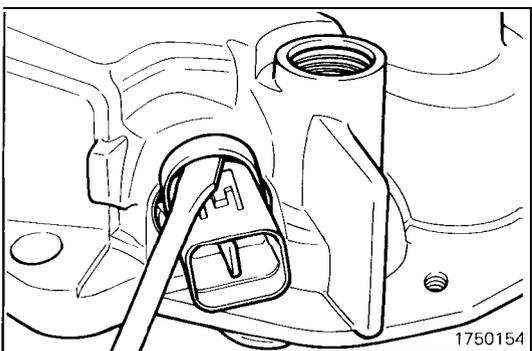
(11) Remove the clip of the solenoid valve connector.
