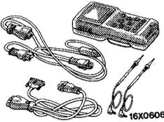
MB991 502 Scan Tool (MUT-II)                    | DRB-II Scan Tool               | Checking the lighting system                   |
