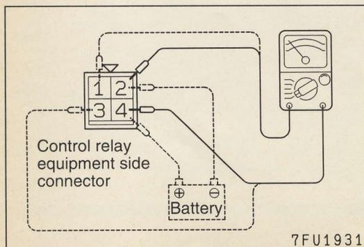
(1) Check for continuity between control relay terminals.
