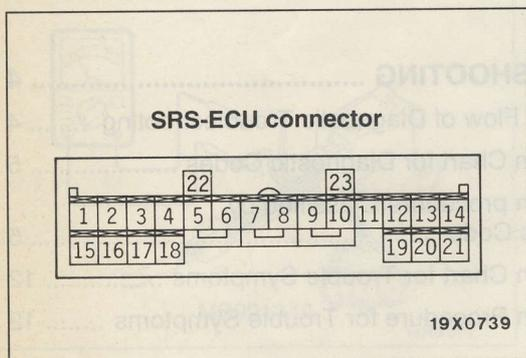
4. Do not attempt to repair the wiring harness connectors of the SRS. If any of the connectors are diagnosed as faulty, replace the wiring harness. If the wires are diagnosed as faulty, replace or repair the wiring harness according to the following table.
