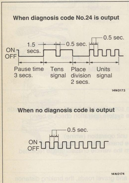
2. Turn the ignition switch to ON and then take a reading of the diagnosis codes from the flashing of the ABS warning lamp.
