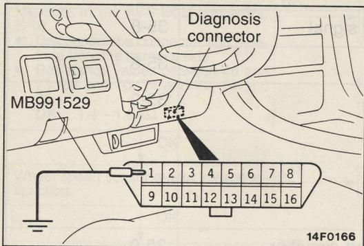
2. Turn the ignition switch to ON and turn the stop lamp switch off and on ten times as shown in the illustration below. Once this has been done, all of the diagnosis codes will be erased.
