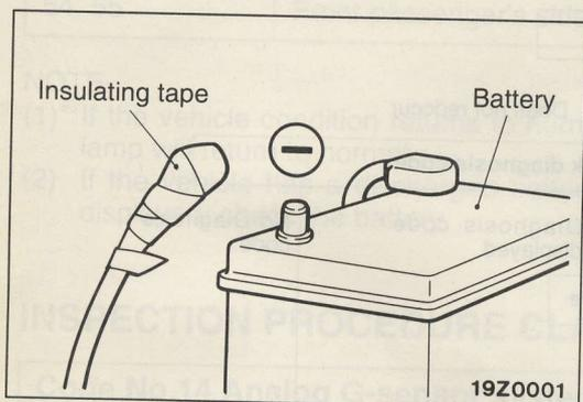
5. After disconnecting the battery cable, wait 60 seconds or more before proceeding with the following work. The SRS system is designed with the following work. The SRS system is designed to retain enough voltage to deploy the air bag for a short time even after the battery has been disconnected, so serious injury may result from unintended air bag deployment if work is done on the SRS system immediately after the battery cables are disconnected.
