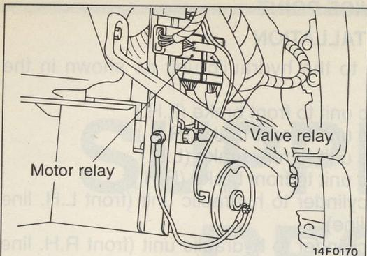
**VALVE RELAY AND MOTOR RELAY CHECK**
