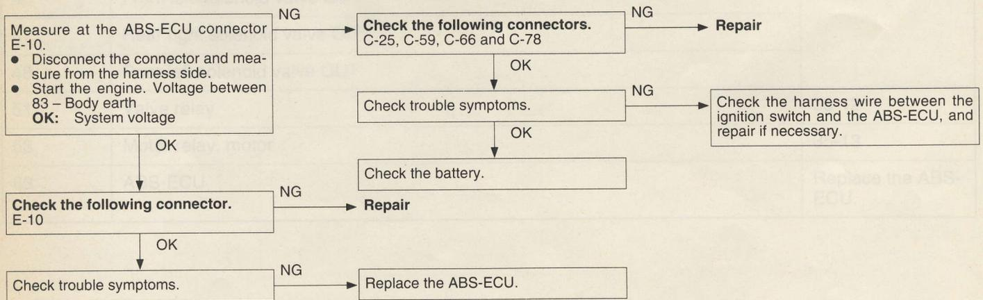
**Code No.21, 22, 23, 24 Wheel speed sensor short circuit**
